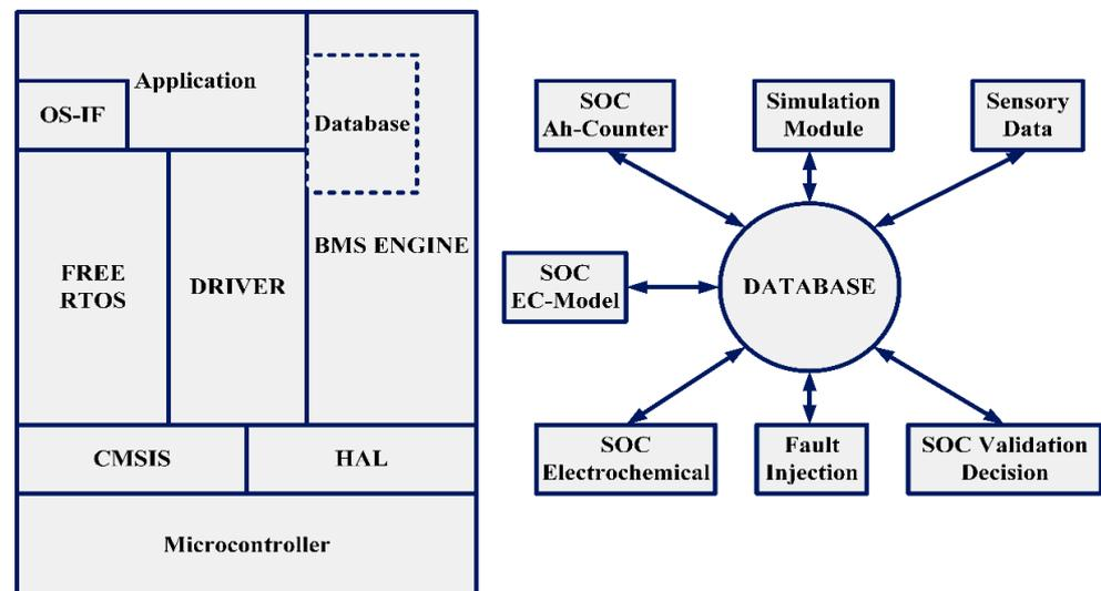
**Figure 3.** BMS software architecture.
