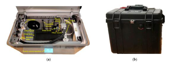
Figure 1. Mark Two 3D printer (desktop series) (a) and dry box to store and supply plastic filaments (b).
