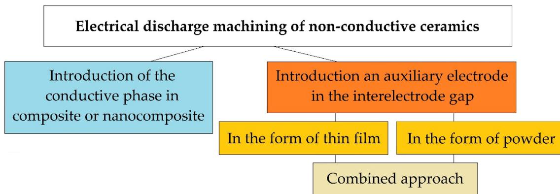
**Figure 2.** Electroerosive methods for processing non-conductive ceramics.
