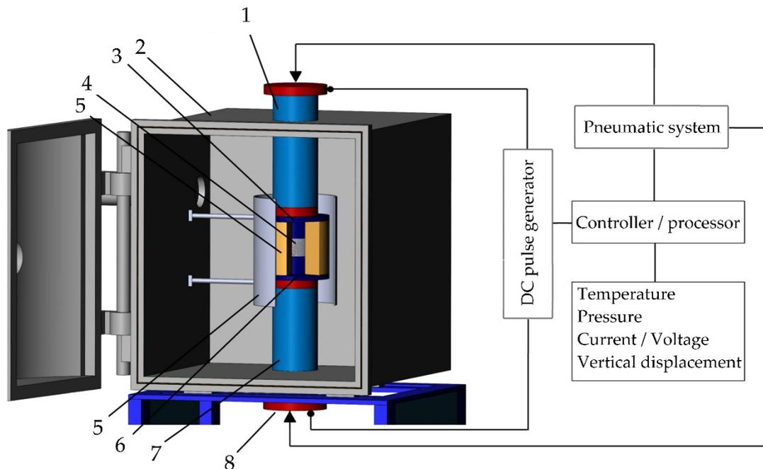
**Figure 6.** The configuration of the spark plasma sintering system developed in MSTU STANKIN: (1) is an upper electrode, (2) is a vacuum chamber, (3) is an upper punch, (4) is pressed powder, (5) is a die block, (6) is a heater, (7) is a lower punch, (8) is a lower electrode.
