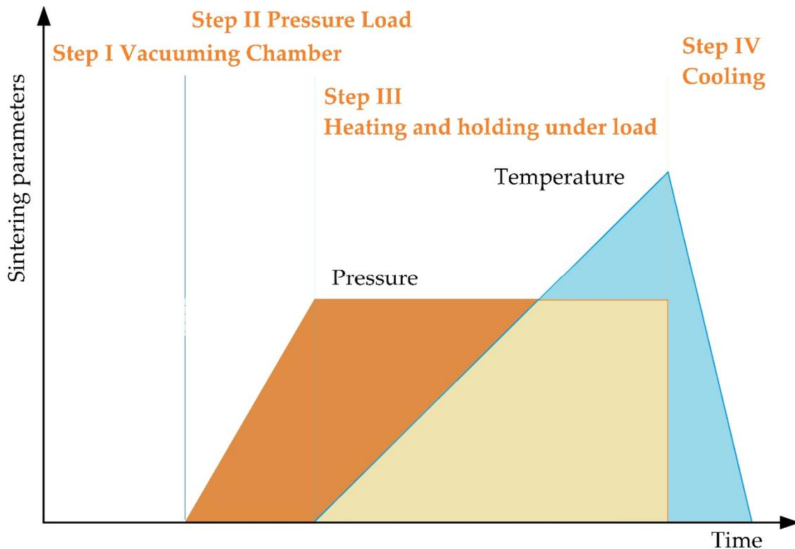
**Figure 7.** The main stages of spark plasma sintering.
