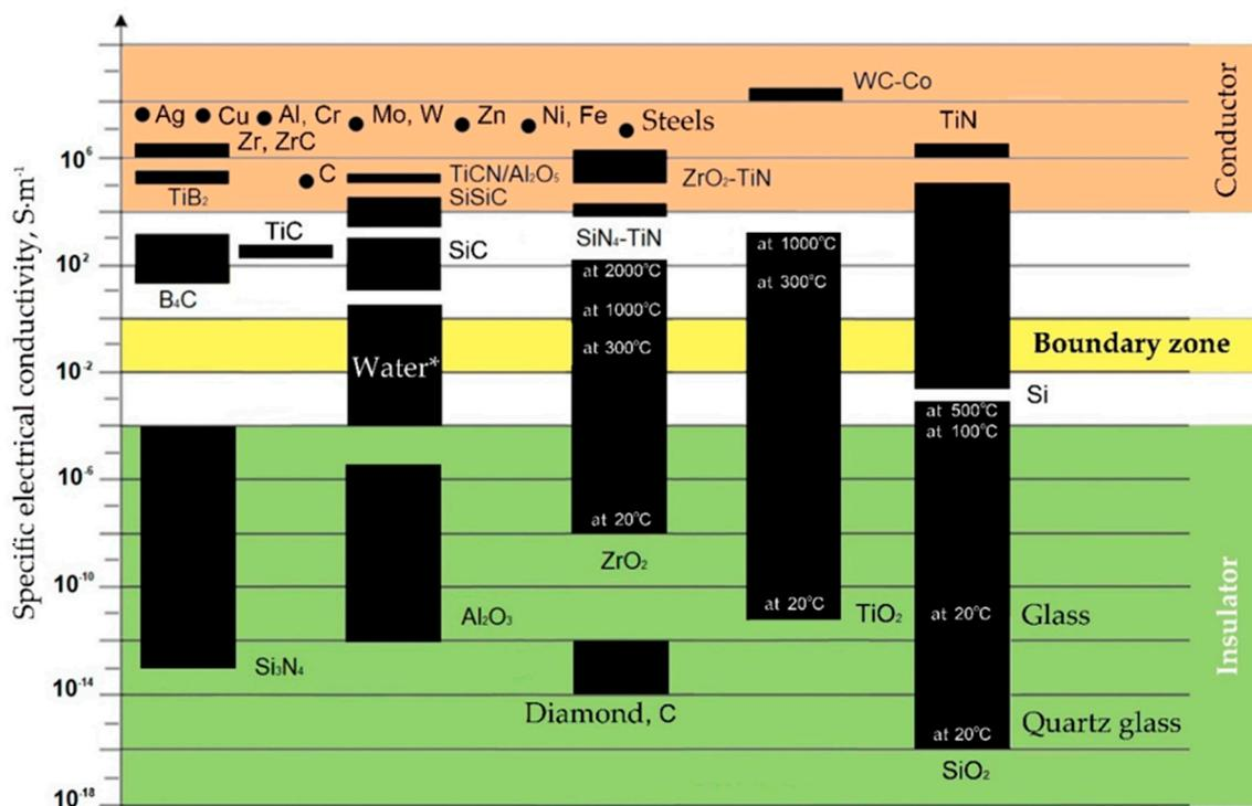
**Figure 3.** Specific electrical conductivity ( $\sigma$ ) of some materials. (\* The electrical conductivity depends on impurities and suspensions, for distilled water is about  $10^{-5} \text{ S}\cdot\text{m}^{-1}$ ).
