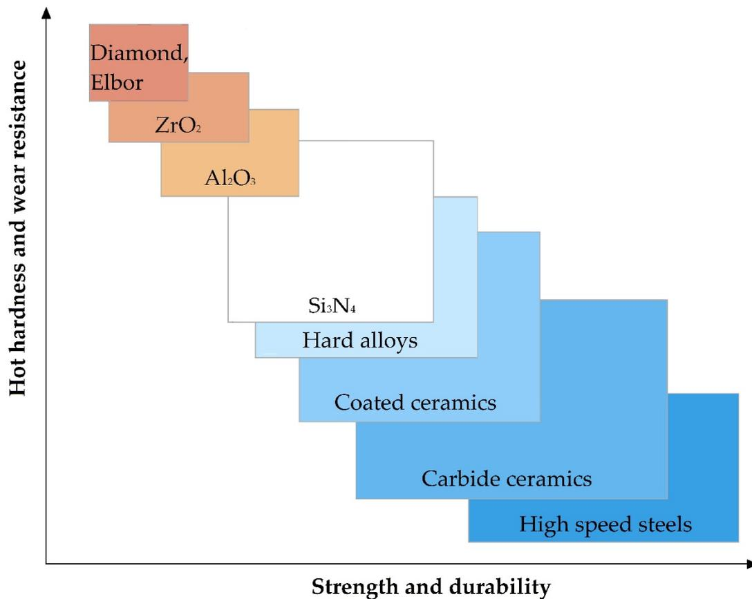
Figure 5. The relationship of the basic physical and mechanical parameters for some materials.
