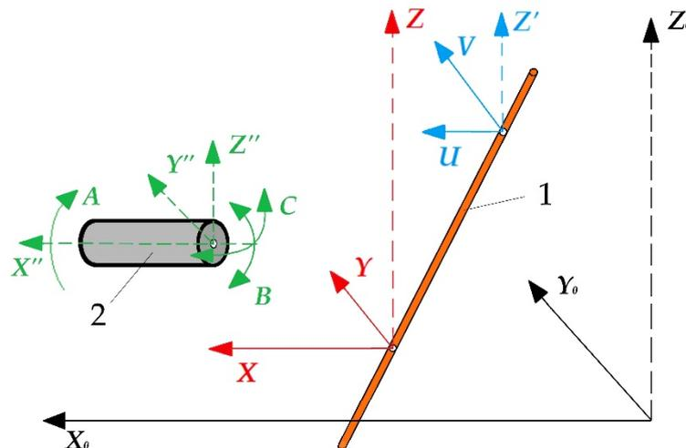
**Figure 1.** Additional rotary axes of wire electrical discharge machining: (1) is a tool, (2) is a part,  $X_0Y_0Z_0$  is an absolute coordinate system of the machine,  $XYZ$  is a relative coordinate system of the lower wire attachment point,  $UVZ'$  is an auxiliary coordinate system of the upper wire attachment point,  $X''Y''Z''$  is a relative coordinate system of the part,  $ABC$  is an additional rotary axes.
