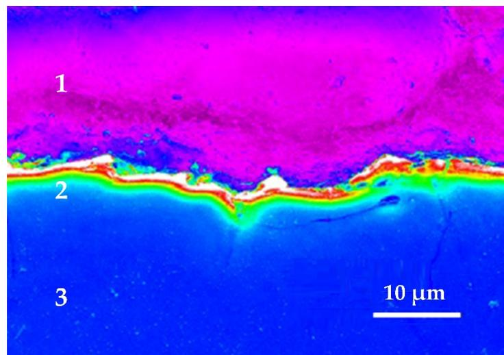
**Figure 4.** White layer obtained by electric discharge machining 99.9% pure chromium by a brass-wire electrode in a water medium: (1) is an epoxy resin that contains a sample for SEM analysis, (2) is a white layer of thermal exposure, a saturated component wire electrode—copper and zinc, (3) is a cut of the machined part made of chromium.
