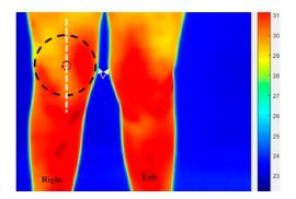
**Figure 1.** A thermal image indicating the manner in which the region of interest (ROI) was selected from the front of the knee. The white line from the center of the circle indicates the height of the ROI. The numerical values on the right-hand side of the figure (i.e., the temperature bar) are temperature values in °C.
