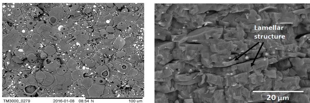
**Figure 11.** (left) Surface morphology of a typical alumina (powder)–YSZ (suspension composite coating) showing multiscale structure [22] and (right) transverse fractured surface of the composite coating showing vertically aligned solidification feature in alumina splats with distributed YSZ (seen as the brighter phase in both micrographs) [21].
