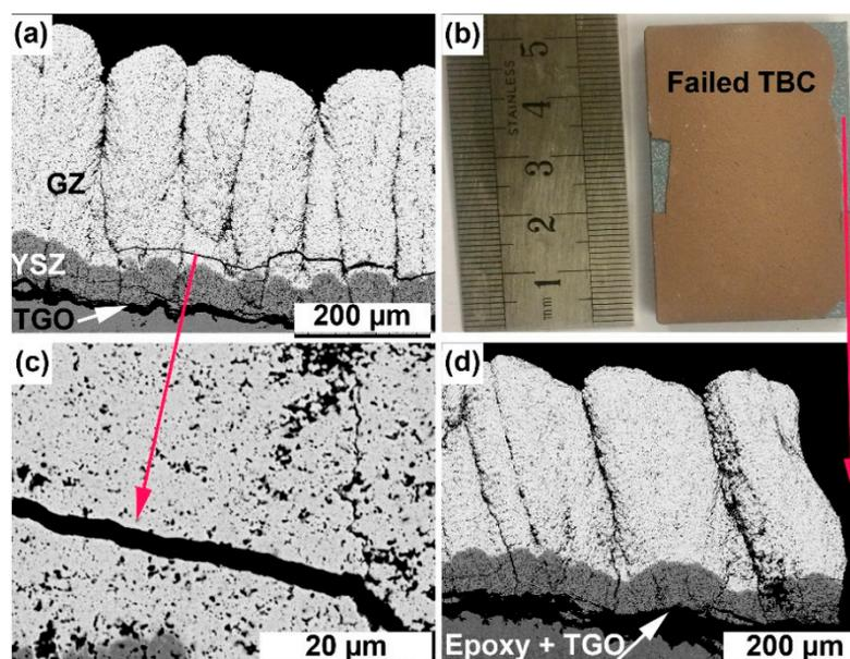
**Figure 7.** A triple layered GZ-based TBC (GZ dense/GZ/YSZ) failed during thermal cyclic fatigue test. (a) SEM micrograph showing failure in TGO; (b) photograph of failed specimen; (c) SEM micrograph showing horizontal crack in GZ; (d) SEM micrograph from different region showing failure in TGO [57]. (GZ = gadolinium zirconate; YSZ = yttria stabilized zirconia; TGO = thermally grown oxide).
