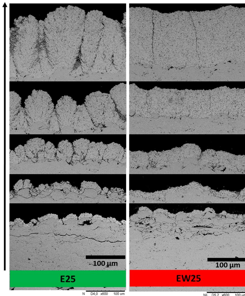
**Figure 8.** Evolution of SPS YSZ microstructure using an ethanol (E25) and ethanol–water (EW25) based suspensions with identical solid loading of 25 wt. %. The former leads to a columnar coating and the latter to a dense vertically cracked coating [49].
