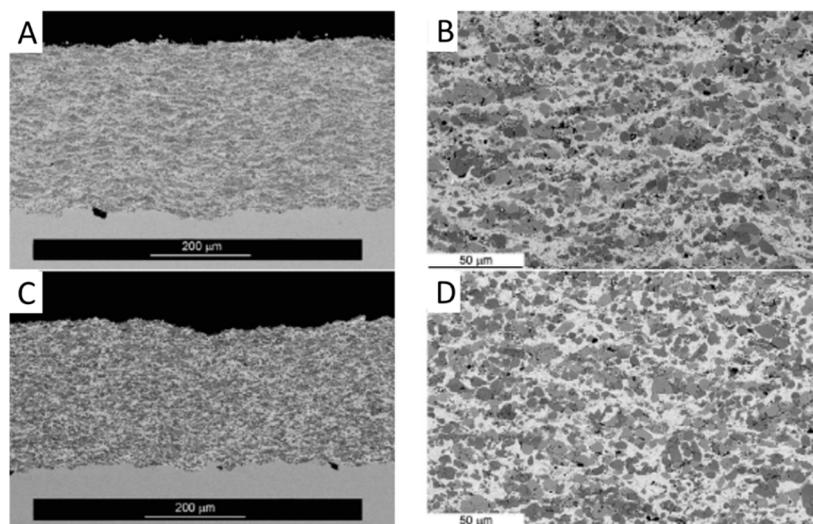
**Figure 2.** (A,C) Low and (B,D) high-magnification micrographs of dense HVOF-sprayed  $\text{Cr}_3\text{C}_2\text{-NiCr}$  coatings, illustrating the ability to refine microstructures by varying nozzle configuration. (A,B): M3; (C,D): M2 [23].
