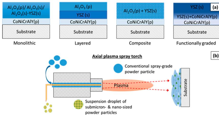
**Figure 10.** (a) Illustration of different coating architectures generated using the hybrid plasma spray setup involving feeding of conventional spray-grade powder (p) and suspension (s) feedstocks as schematically shown in (b) [47].
