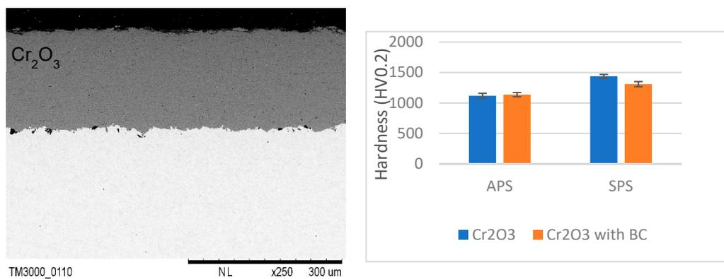
**Figure 9.** Preliminary results with SPS chrome oxide coatings revealing (left) dense coatings with good microstructural integrity and (right) hardness levels that are comparable or exceed those typically achieved by conventional powder-derived plasma spray coatings. (APS = atmospheric plasma spray).
