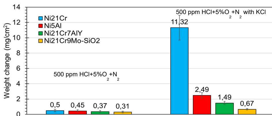
**Figure 4.** Weight change of the HVOF-sprayed Ni<sub>21</sub>Cr, Ni<sub>5</sub>Al, Ni<sub>21</sub>Cr<sub>7</sub>AlY, and Ni<sub>21</sub>Cr<sub>9</sub>Mo-SiO<sub>2</sub> coatings in HCl-laden environment at 600 °C after 168 h exposed with and without KCl.
