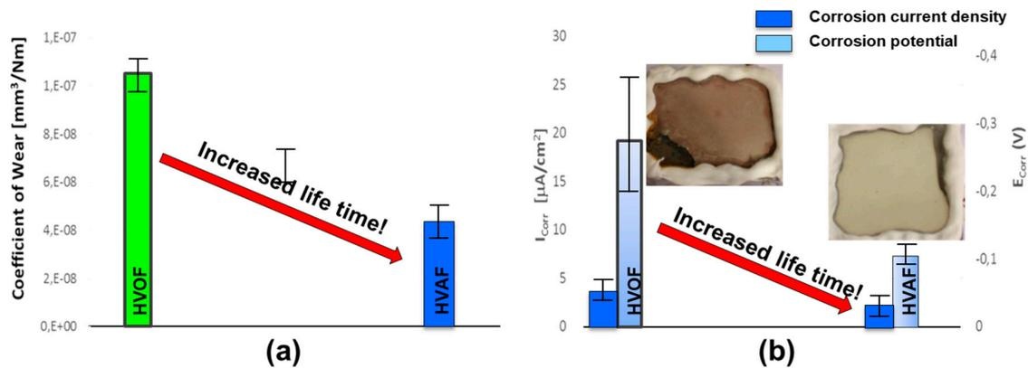
**Figure 3.** Studies showing superior (a) wear and (b) corrosion behavior of HVAF WC-CoCr coatings compared to the corresponding high-velocity oxy-fuel (HVOF) coatings. While (a) depicts the coefficient of wear (in mm<sup>3</sup>/Nm) under abrasive wear conditions, (b) compares the corrosion current density,  $I_{corr}$  (A/cm<sup>2</sup>), and the corrosion potential ( $E_{corr}$ /V) for HVOF and HVAF coatings deposited using identical feedstock.
