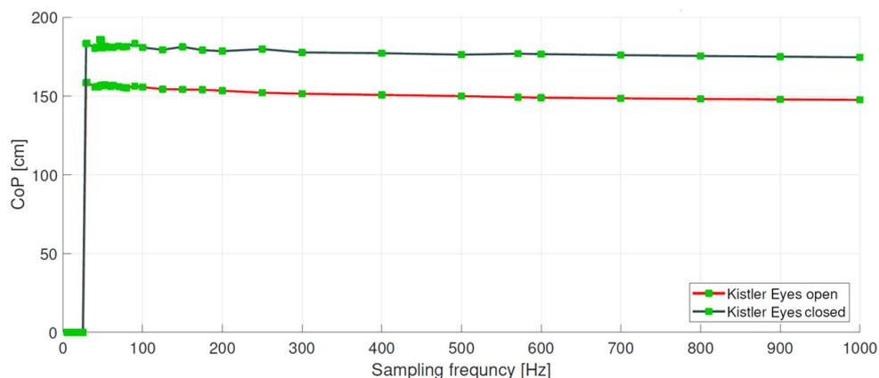
**Figure 6.** Absolute CoP length curve as a function of the sampling frequency used in the bipedal state, with open (EO) and closed eyes (EC), respectively.
