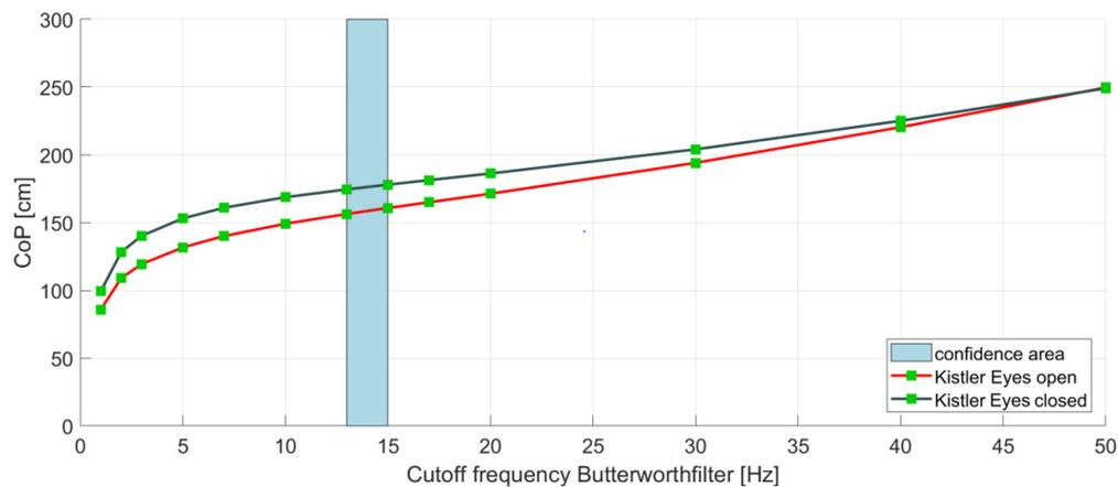
**Figure 8.** Result of the variation of different filter frequencies in the bipedal state for the measurement conditions of eyes open (red) and eyes closed (black).
