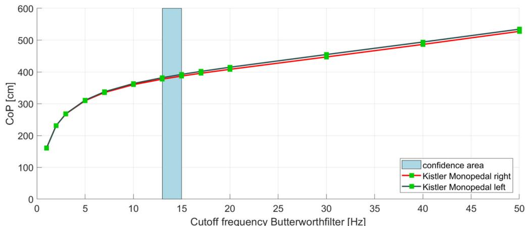
**Figure 9.** Result of the variation of different filter frequencies for the measurement conditions of monopodal left (black) and monopodal right (red).
