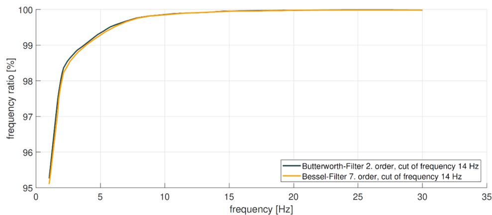
**Figure 11.** Representation of the mean frequency components of the entire spectrum per Hz in percent (blue) after processing the CoP track with a Butterworth second order filter (black) and a Bessel seventh order filter (orange), where the respective cut-off frequency was 14 Hz.
