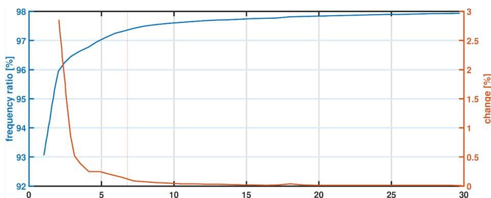
**Figure 10.** Representation of the mean frequency components in the entire spectrum per Hz in percent (blue) and the respective change in frequency per Hz (orange). The red line marks the limit at which the change was less than 0.1%/Hz.
