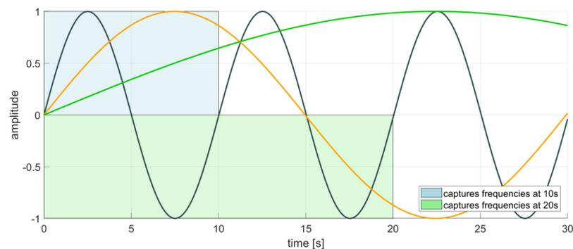
**Figure 2.** Representation of the temporal course of oscillations with different frequencies (0.1 Hz green; 0.01 Hz orange; 0.033 Hz black).
