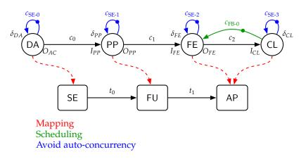
(b) MAPPING B: feature extraction is performed on the smartphone's application processor.
