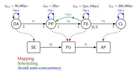
Figure 7. Example CSDF, including mapping and scheduling.
