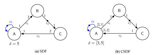
Figure 2. Examples of synchronous dataflow (SDF) and cyclo-static dataflow (CSDF) graphs.
