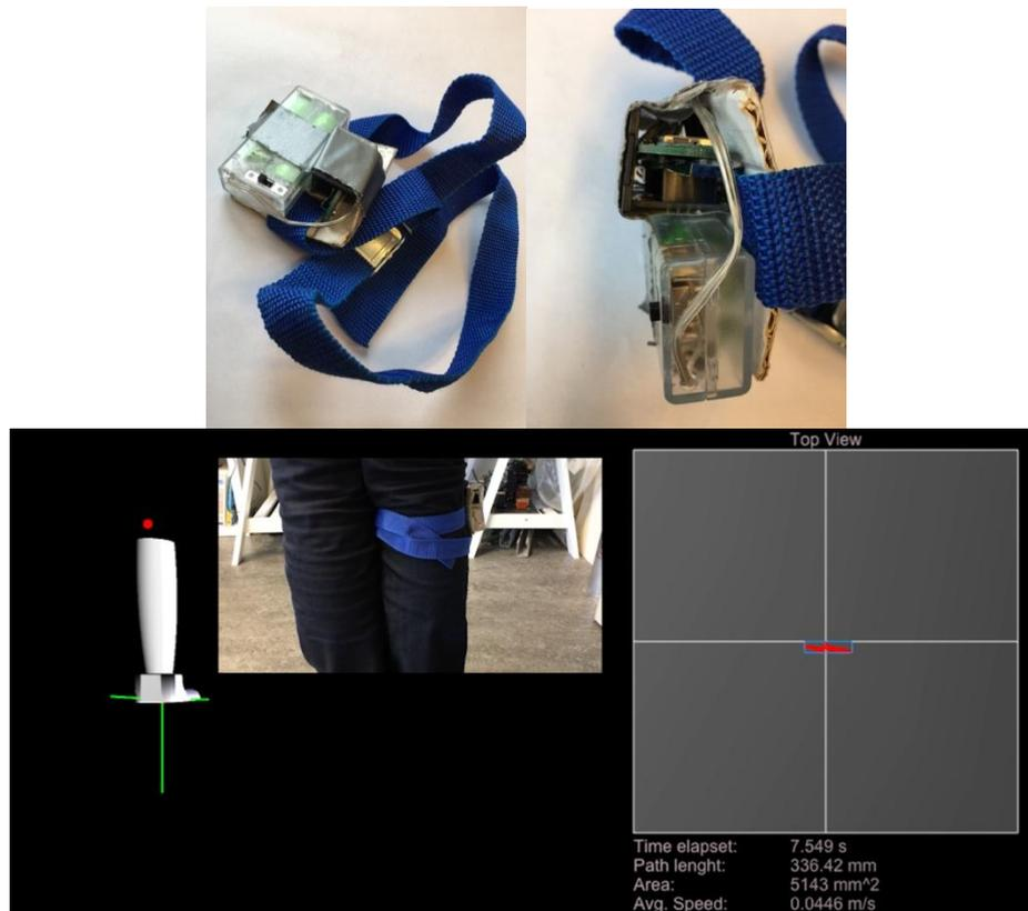
**Figure 1.** External design of the sensor platform of the Arduino prototype and the user interface with visualized (internal) data.
