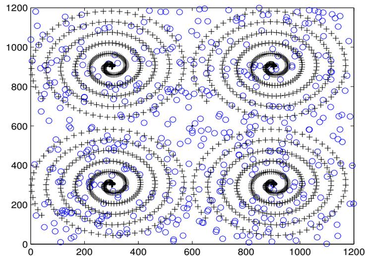
Figure 3. Network design of spiral mobility executed with multiple sinks for large-scale WSNs.
