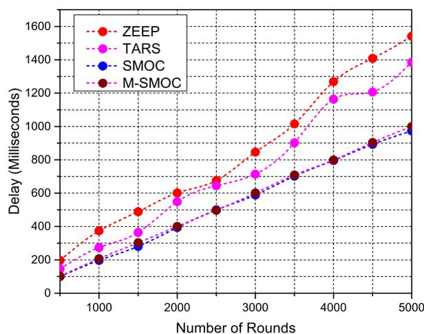
Figure 8. Comparison of the end-to-end delay with respect to the number of rounds.
