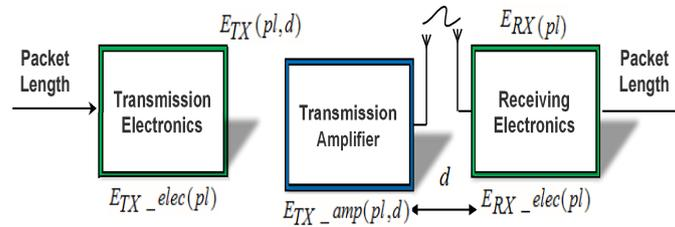
Figure 1. Radio model used in the proposed routing protocols.
