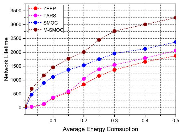
**Figure 6.** Comparison of the network lifetime in terms of energy consumption.
