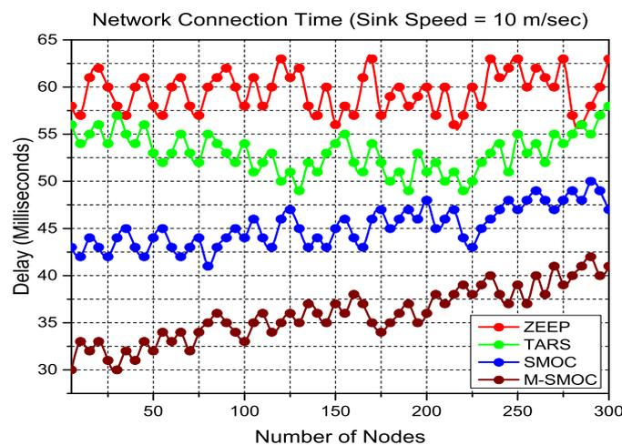
**Figure 12.** Comparison of the network connection time with various sizes of the network.
