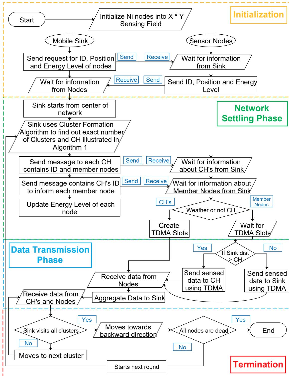
**Figure 4.** Flowchart of the proposed Spiral Mobility based on Optimized Clustering (SMOC) and Multiple sink-based SMOC (M-SMOC) routing protocols.
