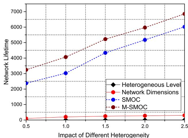
**Figure 14.** Comparison of the network lifetime of the proposed protocols with various sizes of networks.
