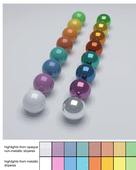
Figure 2. Image of spheres modeled and rendered with the RADIANCE software, showing the colors of highlights present in non-metallic and metallic materials with the same spectral reflectance.
