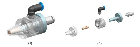
Figure 1. (a) New nozzle solution assembly; (b) exploded diagram of the nozzle.
