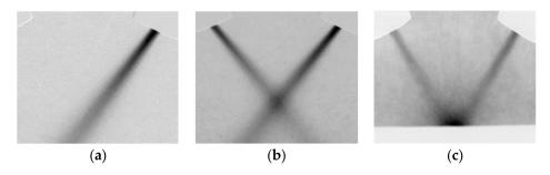
**Figure 3.** (a) One active nozzle; (b) two active nozzles; (c) two active nozzles with a substrate at 15 mm.
