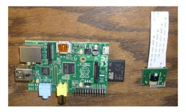
Figure 5. Raspberry Pi and camera.
