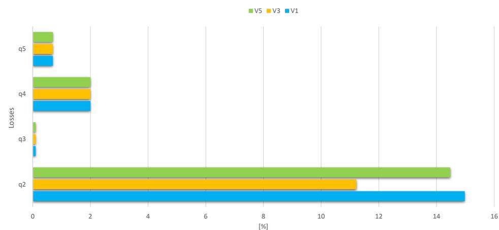
**Figure 3.** Energy losses by the indirect method for the G.V. type VU-40.
