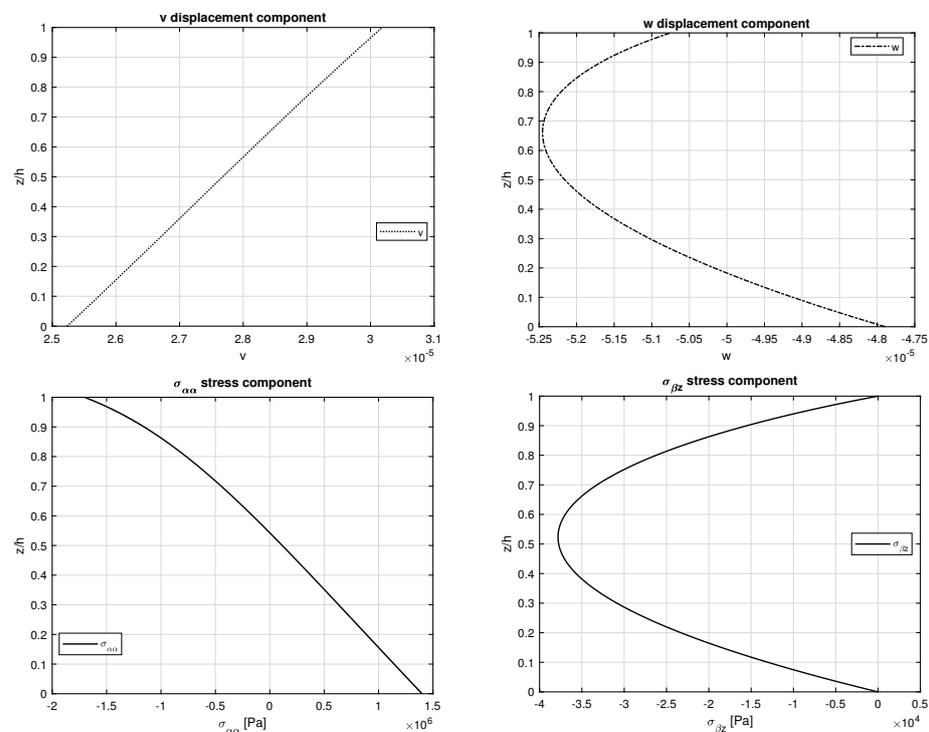
Figure 7. Second benchmark, displacements and stresses for a thick ( $R_\alpha/h = 10$ ) simply supported cylinder with one FGM ( $p = 1$ ) layer obtained using the 3D-u- $\theta$  model. Maximum amplitudes:  $w$  and  $\sigma_{\alpha\alpha}$  at  $(a/2, b/2)$ ;  $v$  and  $\sigma_{\beta z}$  at  $(a/2, 0)$ .
