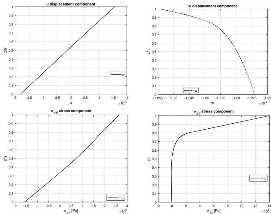
**Figure 10.** Third benchmark, displacements and stresses for a thick ( $R_\alpha/h = 10$ ) simply supported sandwich cylindrical shell with FGM ( $p = 2$ ) core obtained using the 3D-u- $\theta$  model. Maximum amplitudes:  $w$  and  $\sigma_{\beta\beta}$  at  $(a/2, b/2)$ ;  $u$  at  $(0, b/2)$ ;  $\sigma_{\alpha\beta}$  at  $(0, 0)$ .
