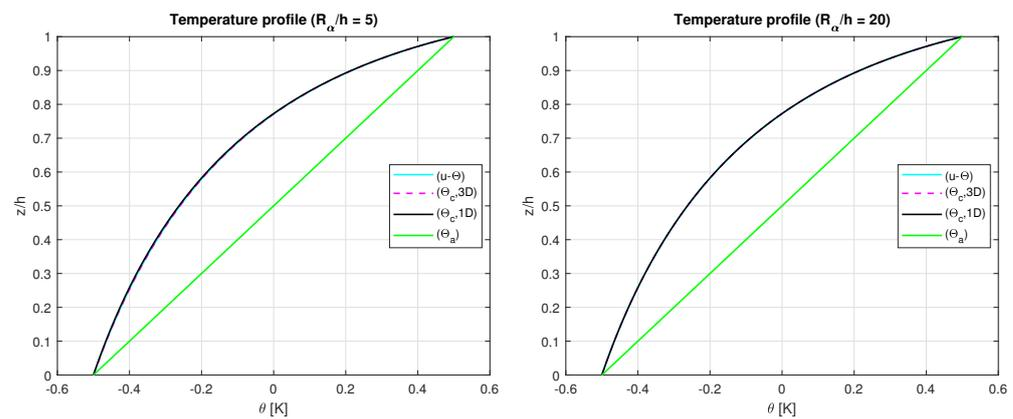
**Figure 6.** Second benchmark, temperature profiles for thick and moderately thick simply supported cylinders with one FGM ( $p = 1$ ) layer. The maximum amplitude of the temperature  $\theta(\alpha, \beta, z)$  is evaluated at the centre of the cylinder ( $a/2, b/2$ ).
