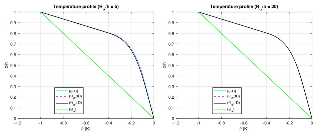
**Figure 9.** Third benchmark, temperature profiles for thick and moderately thick simply supported sandwich cylindrical shells with FGM ( $p = 2$ ) core. The maximum amplitude of the temperature  $\theta(\alpha, \beta, z)$  is evaluated at the centre of the cylindrical shell at  $(a/2, b/2)$ .
