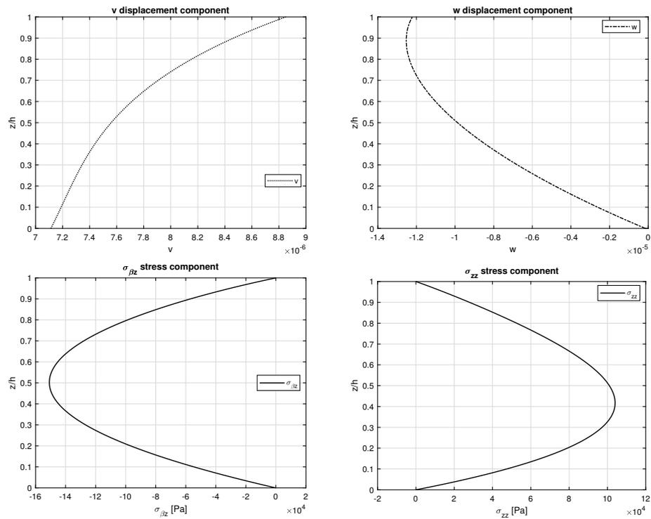
**Figure 13.** Fourth benchmark, displacements and stresses for a thick ( $R_\alpha/h = 10$ ) simply supported spherical shell with one FGM ( $p = 2$ ) layer obtained using the 3D-u- $\theta$  model. Maximum amplitudes:  $w$  and  $\sigma_{zz}$  at  $(a/2, b/2)$ ;  $v$  and  $\sigma_{\beta z}$  at  $(a/2, 0)$ .
