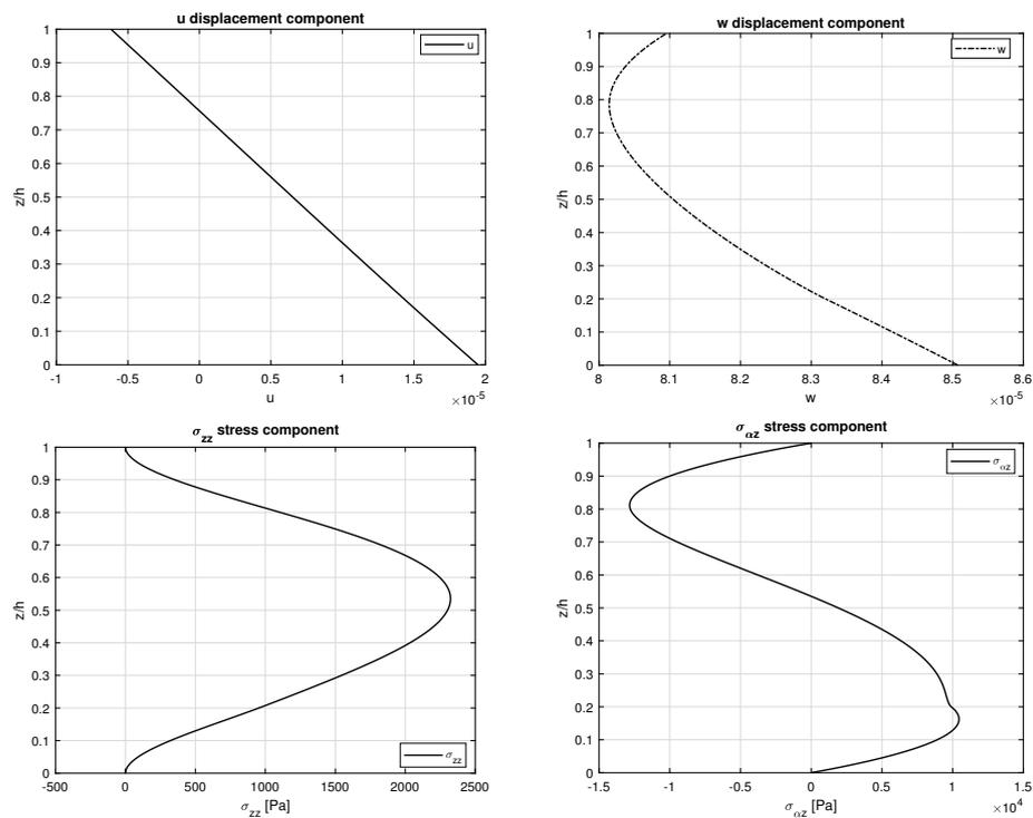
**Figure 4.** First benchmark, displacements and stresses for a thick ( $a/h = 10$ ) simply supported sandwich square plate with FGM ( $p = 0.5$ ) core obtained via the 3D-u- $\theta$  model. Maximum amplitudes:  $w$  and  $\sigma_{zz}$  at ( $a/2, b/2$ );  $u$  and  $\sigma_{\alpha z}$  at ( $0, b/2$ ).
