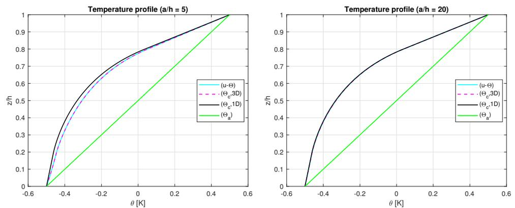
**Figure 3.** First benchmark, temperature profiles for thick and moderately thick simply supported sandwich square plates with FGM ( $p = 0.5$ ) core. The maximum amplitude of the temperature  $\theta(\alpha, \beta, z)$  is evaluated at the centre of the plate ( $a/2, b/2$ ).
