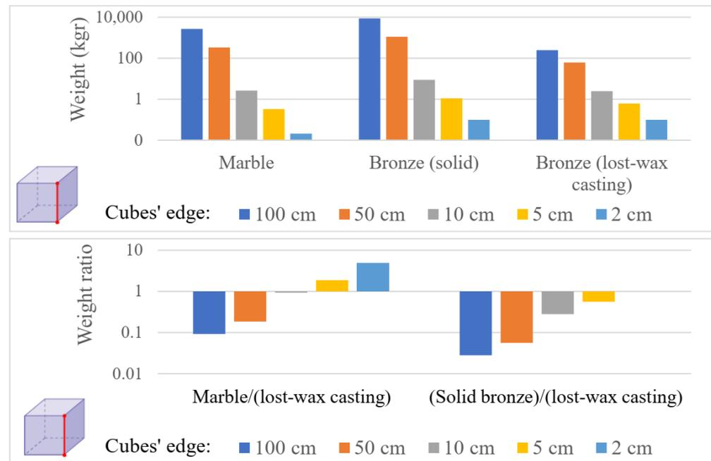
**Figure 6.** Top: The weight of cubes made from marble, solid bronze or bronze with the lost-wax casting process with different edges; bottom: the weight ratio between different techniques (four faces).
