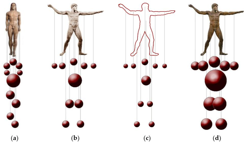
**Figure 7.** Analysis of forms and forces in Ancient Greek sculpture: (a) massive marble, carving method: Kouros c. 530 BC; (b) massive marble, simulation of Poseidon of Artemision c. 460 BC; (c) lost-wax casting (as created) of Poseidon of Artemision c. 460 BC (section of the statue represents lost-wax casting method); (d) massive bronze, Poseidon of Artemision c. 460 BC (statue figures adapted from [27,28]).
