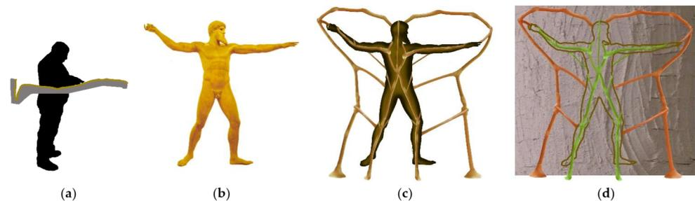
**Figure 4.** Basic steps of lost-wax casting method: (a) a craftsman makes the wax model; (b) wax model shell; (c) network of wax tubes inside (for the outgoing of the wax in green) and outside (for the entry of metal); (d) enclosing of the wax model (including the wax-tubes network) in fire-resistant mortar.
