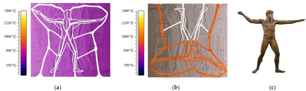
**Figure 5.** Basic steps of lost-wax casting method: (a) the fire-resistant mortar with the wax model and wax-tubes network is heated to 250–350 °C for 3–15 days (depending on the size of statue) and the wax is melted out; (b) metal foundry; (c) final artifact after the removal of metal tubes.
