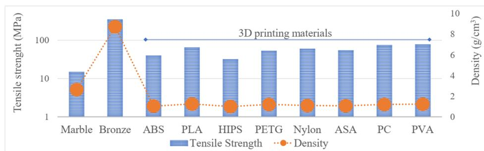
**Figure 11.** Evaluation of marble, bronze and common 3D printing materials. ABS: acrylonitrile butadiene styrene; PLA: polylactic acid; HIPS: high impact polystyrene; PETG: glycolized polyester; ASA: acrylonitrile styrene acrylate; PC: polycarbonate; PVA: polyvinyl alcohol.
