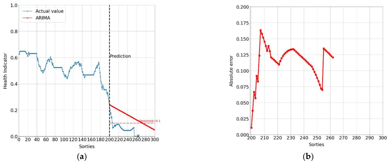
Figure 13. Prediction of the landing gear HI for Plane #5: (a) results and (b) absolute error of estimated twenty sorties.
