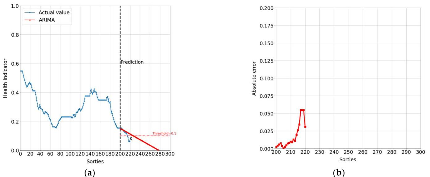
**Figure 11.** Prediction of the landing gear HI for Plane #3: (a) results and (b) absolute error of estimated twenty sorties.
