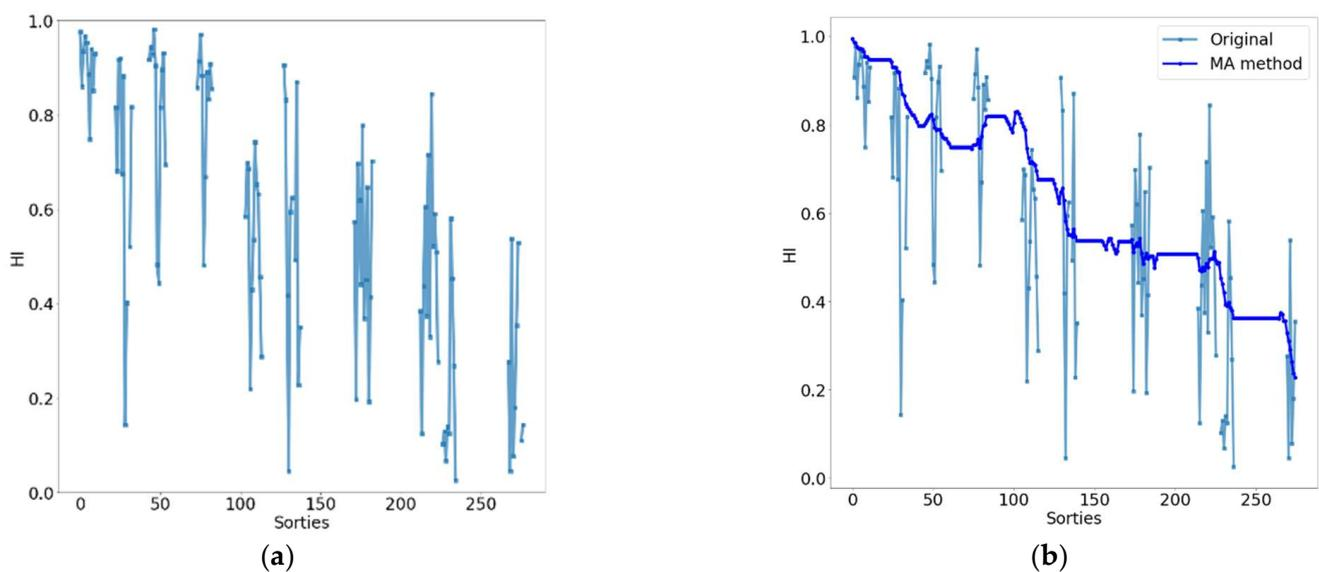
Figure 8. Landing gear's HI: (a) original and (b) with missing data imputed using the moving average method.
