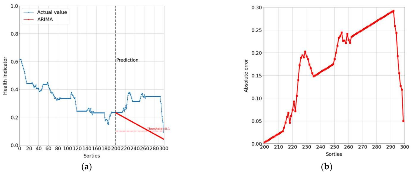
**Figure 10.** Prediction of the landing gear HI for Plane #2: (a) results and (b) absolute error of estimated twenty sorties.
