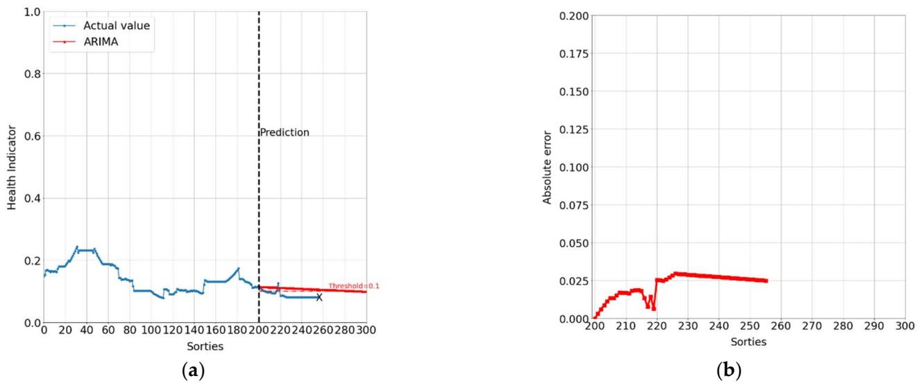
Figure 12. Prediction of the landing gear HI for Plane #4: (a) results and (b) absolute error of estimated twenty sorties.
