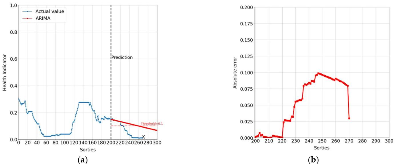
**Figure 9.** Prediction of the landing gear HI for Plane #1: (a) results and (b) absolute error of estimated twenty sorties.
