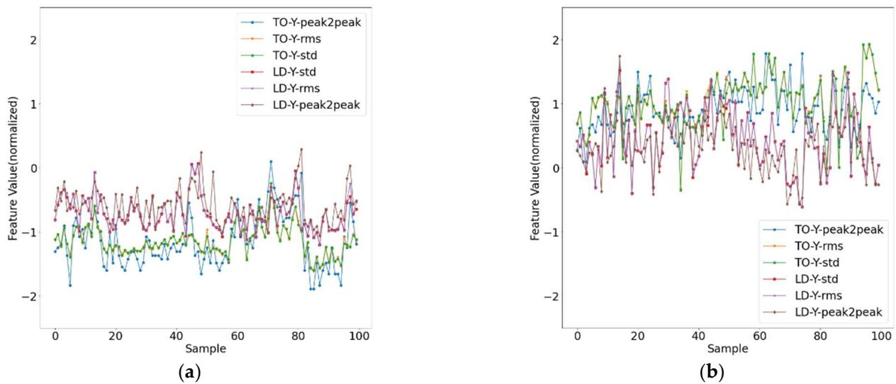
Figure 5. Top six ranking features from the vibration signal: (a) healthy and (b) faulty.
