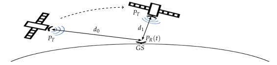
Figure 1. Communication link early in an overflight and close to the zenith.
