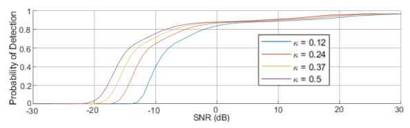
Figure 7. Detector performance for simulated satellite signal in an ISM environment.
