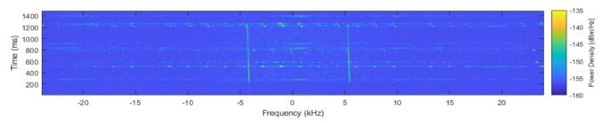
Figure 3. Spectrogram of satellite burst from 0.23 to 1.23 s received at GS close to the zenith.
