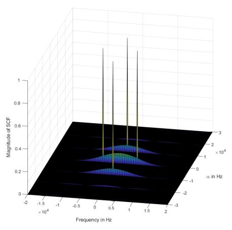
**Figure 4.** Spectral correlation function (SCF) of a Gaussian frequency-shift keying (GFSK) modulated signal with a symbol rate of  $f_s = 9600 \frac{\text{symbols}}{\text{second}}$  and a center frequency of  $f_0 = 0$  Hz.
