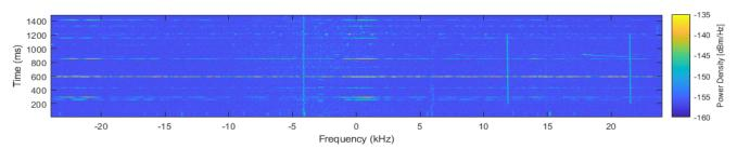
Figure 2. Spectrogram of satellite burst from 0.23 to 1.23 s received at ground station (GS) early in an overflight.
