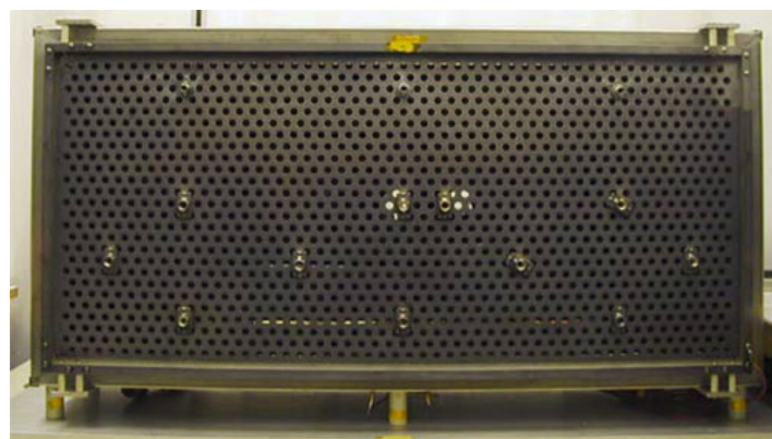
Figure 15. The discharge chamber of the HiPEP ion thruster developed for the nuclear-powered Jupiter Icy Moons Orbiter.
