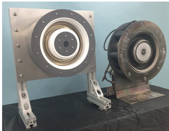
Figure 9. The H9 (left), a 9 kW magnetically-shielded Hall thruster, and the H6 (right), a 6 kW unshielded Hall thruster. Both were developed by the Jet Propulsion Laboratory, the Air Force Research Laboratory, and the University of Michigan.
