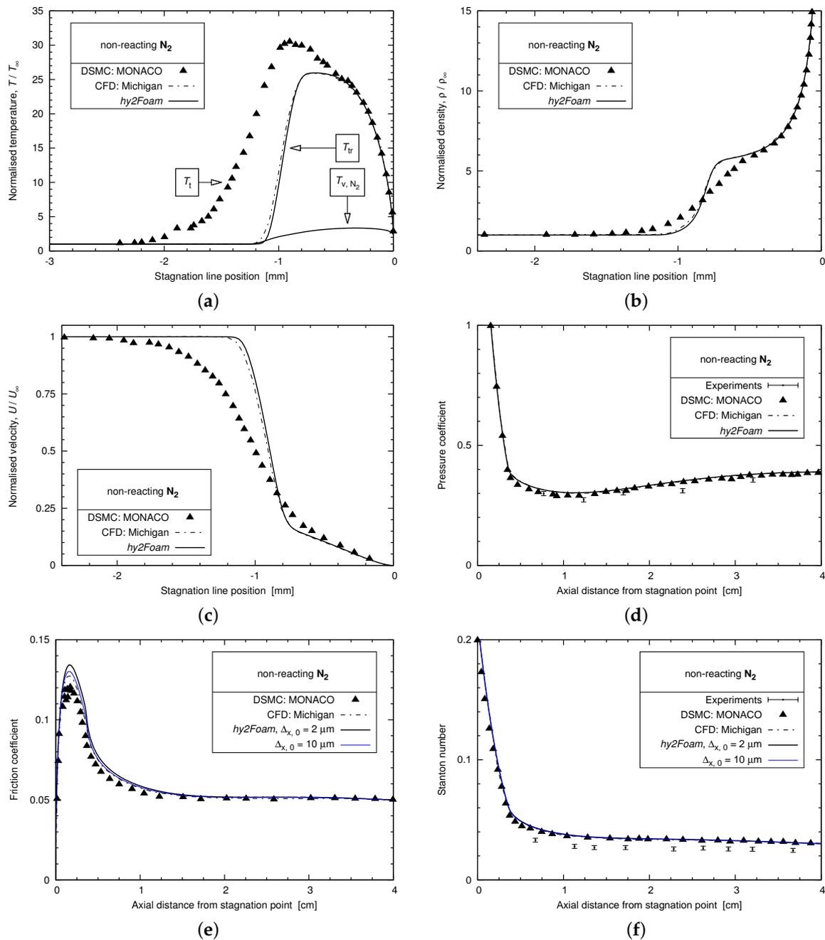
**Figure 2.** (a–c) Stagnation line profiles, and (d–f) surface quantities along the blunted cone; (a) normalised temperature; (b) normalised mass density; (c) normalised velocity; (d) pressure coefficient; (e) friction coefficient; (f) Stanton number.
