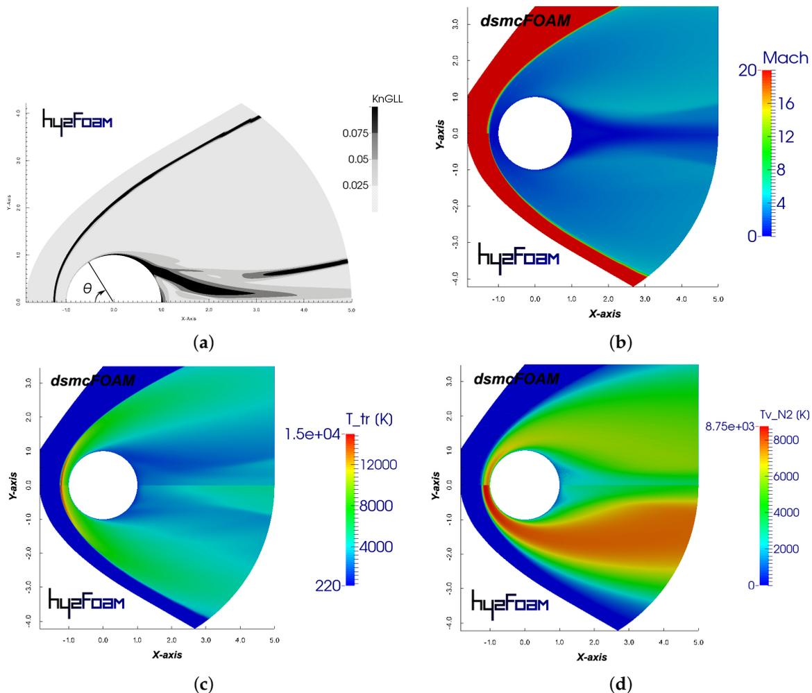
**Figure 4.** Computational fluid dynamics-direct simulation Monte Carlo (CFD-DSMC) flow-field comparisons for run number 2. In (b–d): the *dsmcFoam* solution is represented in the upper half and the *hy2Foam* solution in the lower half. (a) Local gradient-length Knudsen number; (b) Mach number; (c) trans-rotational temperature; and (d) vibrational temperature.
