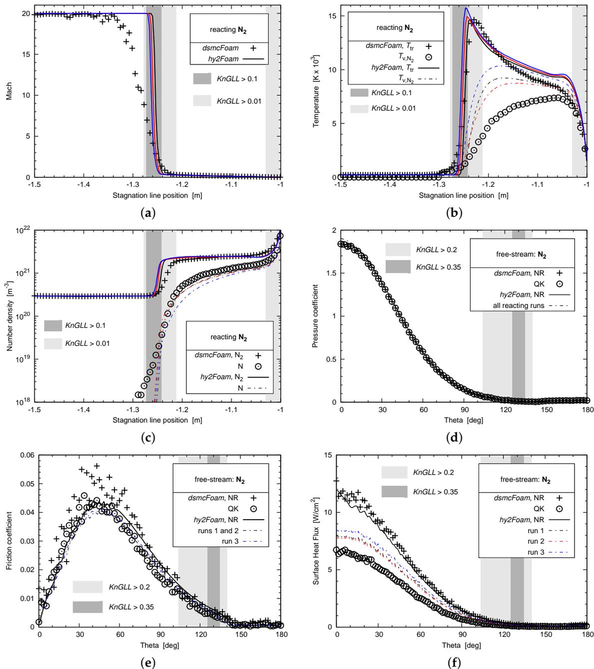
**Figure 5.** (a–c): Stagnation line profiles. CFD run 1: **black lines**, run 2: **red lines**, run 3: **blue lines**. (d–f): surface quantities around the cylinder. (a) Mach number; (b) temperature; (c) number density; (d) pressure coefficient; (e) skin-friction coefficient; (f) surface heat flux.
