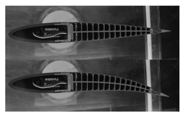
**Figure 3.** FishBAC wind tunnel test model showing baseline and morphed shapes.
