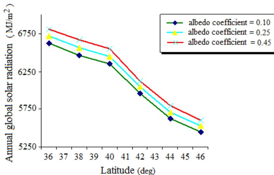
**Figure 2.** Annual global solar radiation as a function of latitude and three albedo values, collected by a typical surface with a tilt angle of  $\beta = 35^\circ$ . The green, turquoise and red lines refer to the annual solar radiation collected on the surface as a function of the albedo values  $\rho = 0.10$  (conifer forest),  $\rho = 0.25$  (green grass) and  $\rho = 0.45$  (desert sand), respectively.
