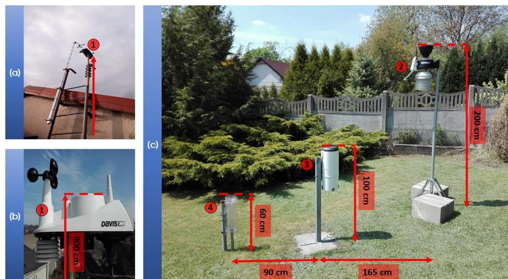
**Figure 3.** Location of rain gauges: (a,b) 1—Davis Vantage Vue rain gauge, (c) 2—Davis Vantage Pro 2A rain gauge, (c) 3—Hellmann rain gauge, (c) 4—Stratus rain gauge.
