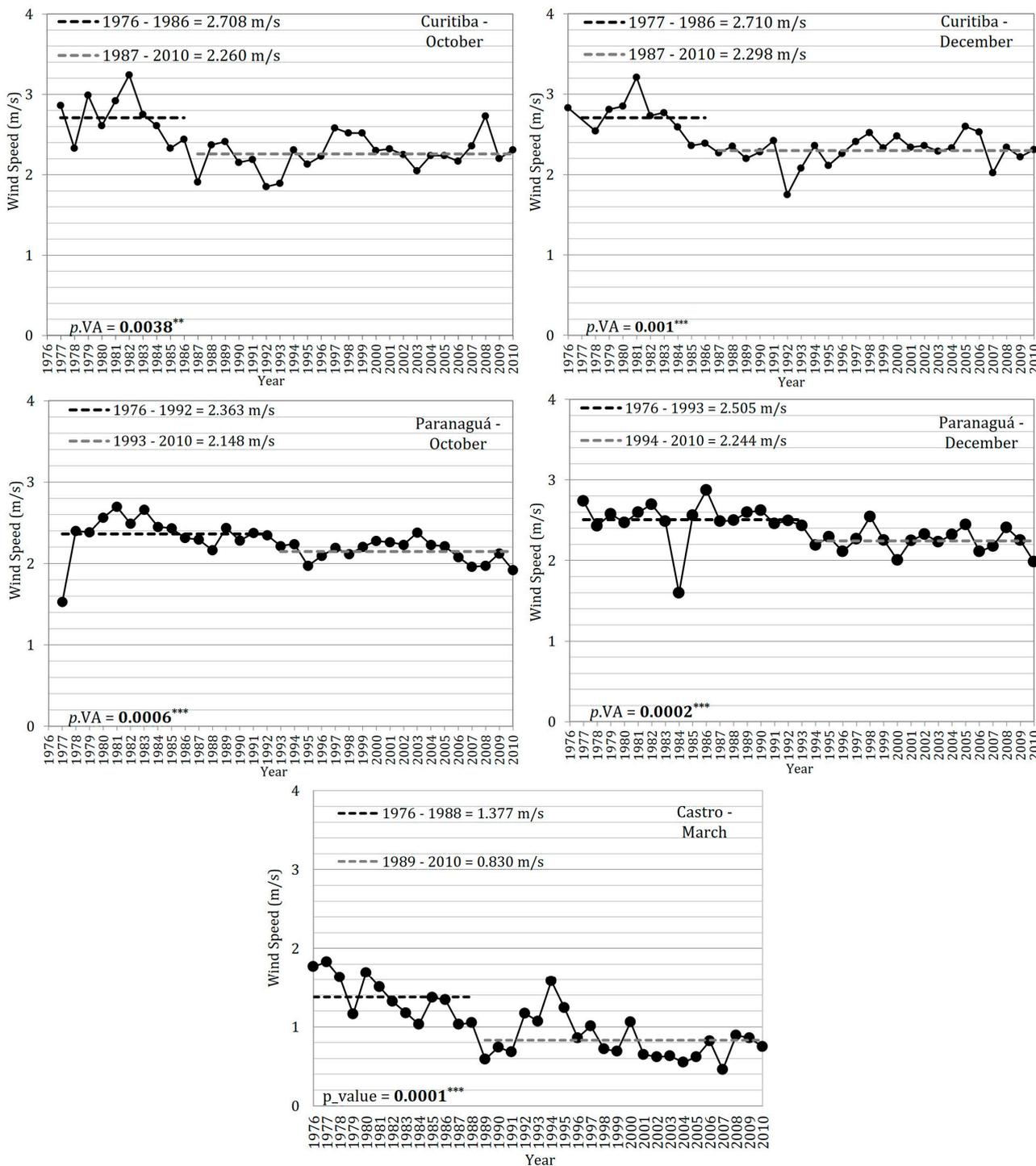
**Figure 7.** Representation of ruptures (Pettitt test) verified in time series of seasonal wind speed (m/s) in Curitiba and Paranaguá (Paraná, Brazil). Legend: \*\*\* = 99.9% significance; \*\* = 99% significance;  $p.VA$  = significance level. In bold the results with statistical significance.
