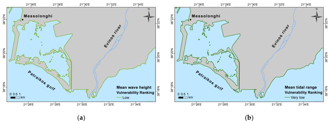
**Figure 4.** Assigned vulnerability classes in response to (a) mean wave height and (b) mean tidal range.
