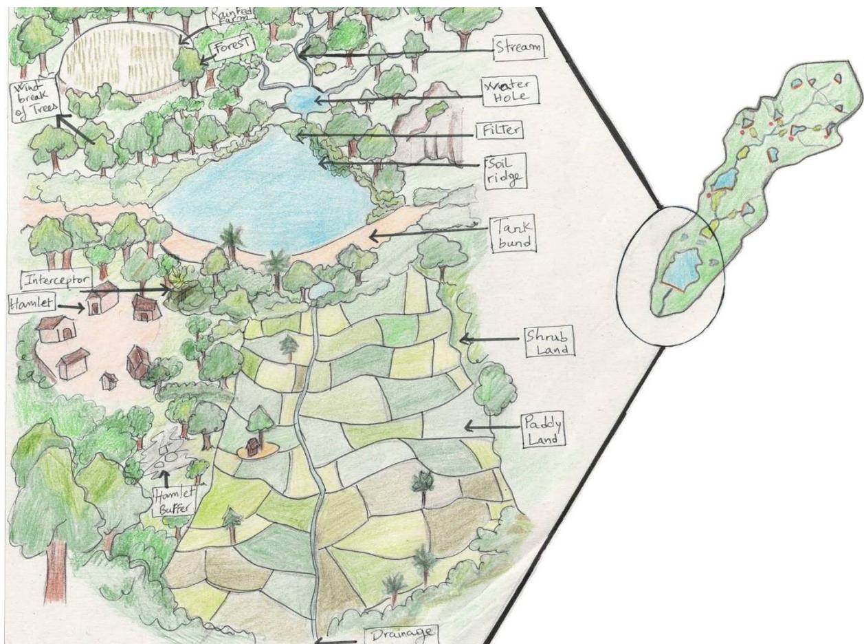
Figure 1. Main components of the tank.
