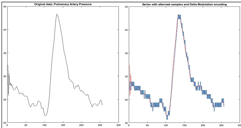
**Figure 5.** Delta modulation (DM) encoding for pulmonary artery pressure biosensor.
