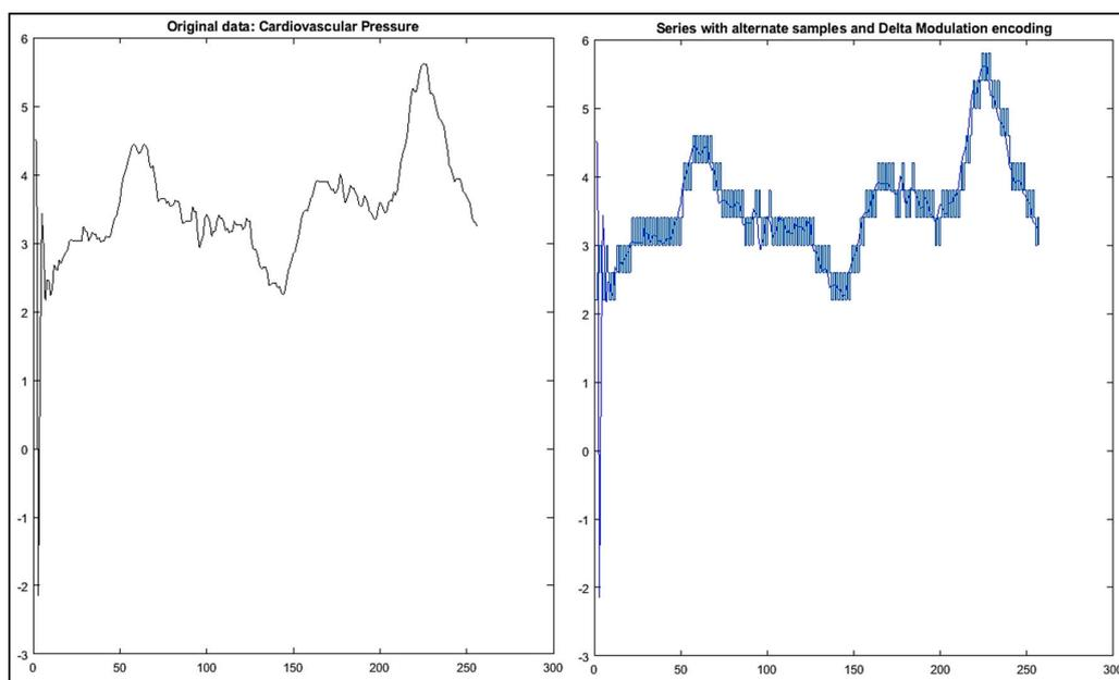
**Figure 6.** DM encoding for cardiovascular pressure biosensor.
