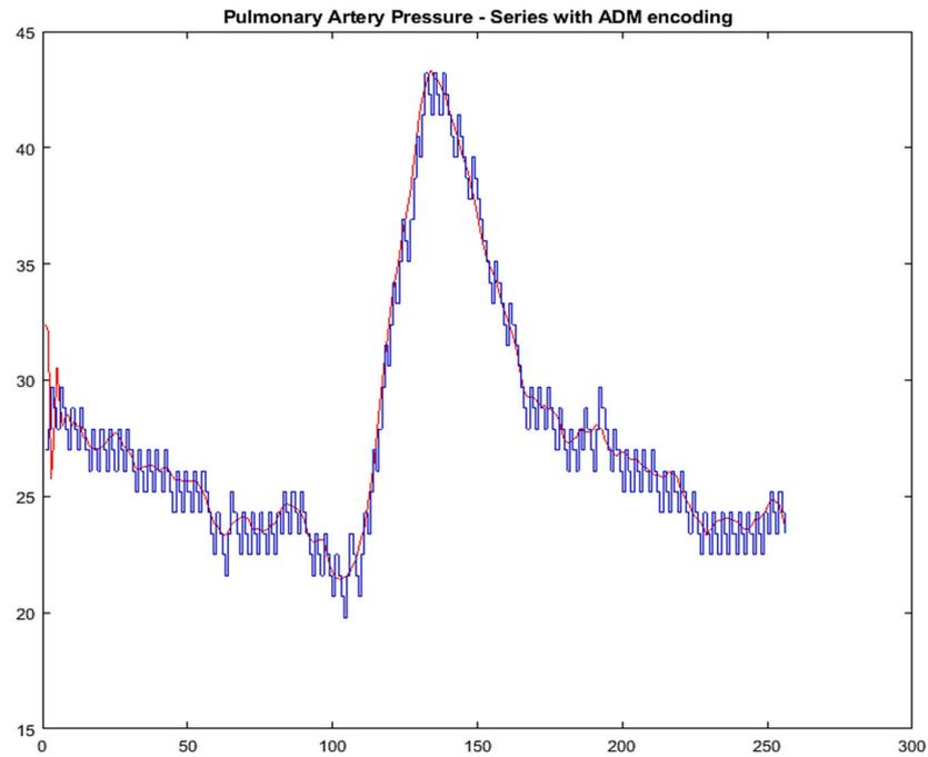
**Figure 7.** Adaptive delta modulation (ADM) encoding for pulmonary artery pressure biosensor.
