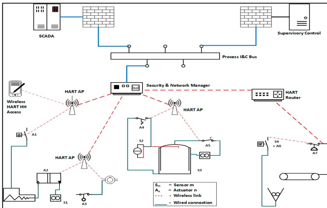
**Figure 1.** A WirelessHART (Wireless Highway Addressable Remote Transducer)-based network with sensors and actuators.
