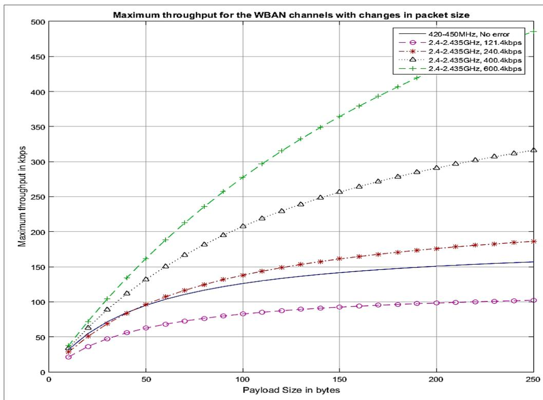
Figure 11. Maximum throughput vs. the payload in bytes.
