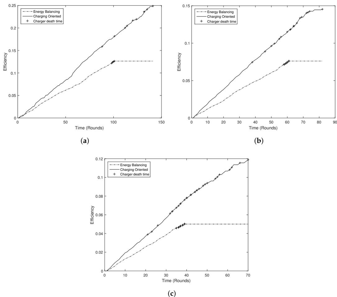
**Figure 5.** Cumulative charging efficiency over time for (a) 10, (b) 20 and (c) 30 chargers respectively.
