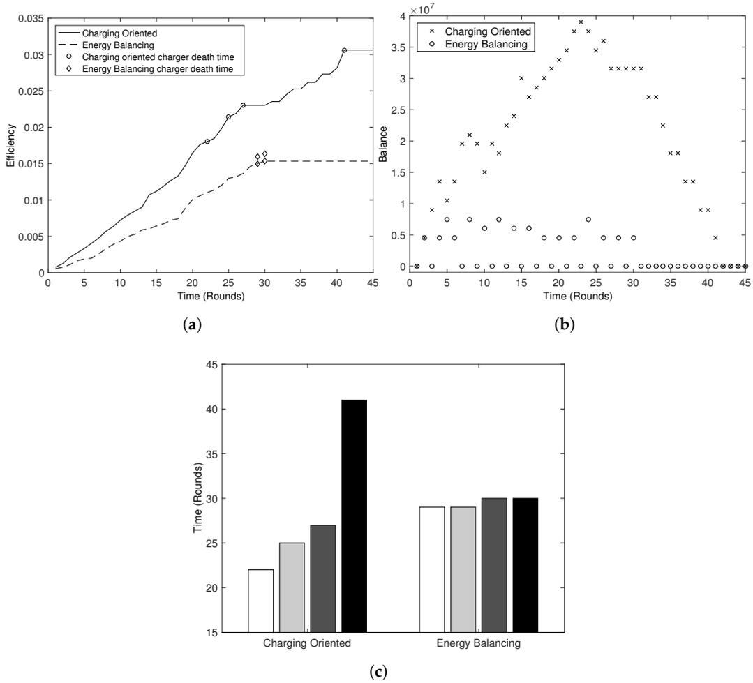
**Figure 2.** Experimental evaluation of the various metrics. (a) Cumulative charging efficiency over time. (b) Energy balance over time. (c) Lifetime of the chargers.
