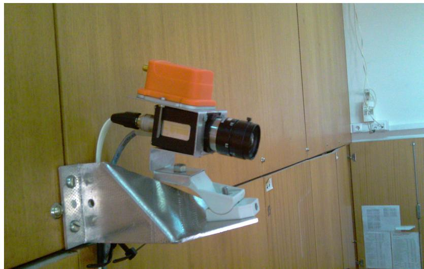
**Figure 9.** Experimental setup for a smart sensor. AVT Prosilica GC650C camera coupled with a Xsens MTx inertial sensor mounted on the wall. We setup a network of these smart sensors around the room (Videos are available at YouTube <https://www.youtube.com/watch?v=rPibqw4cAxc> or in the Supplementary file and more details are available at the website: <http://sites.google.com/site/hdakbarpour/research>).
