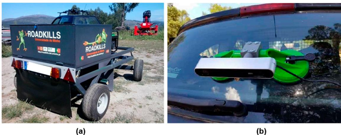
**Figure 1.** Image of: (a) the mobile mapping system 1 (MMS1) outdoors and (b) the mobile mapping system 2 (MMS2) attached to the back of a vehicle. The complete MMS2 system also includes a laptop and a lighter charger that go inside the vehicle.
