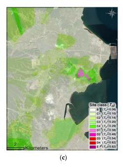
**Figure 6.** Seismic zonation for geotechnical response-parameter-based, site-specific effects: (a) H; (b)  $V_{S30}$ ; (c)  $T_G$ .
