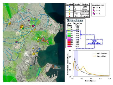
**Figure 9.** Spatial comparison between  $T_G$ -based seismic zonation and earthquake damage category of buildings.
