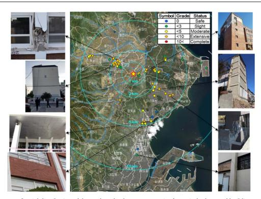
**Figure 8.** Spatial distribution of the earthquake damage categories for majorly damaged buildings and images of buildings.
