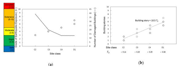
**Figure 10.** Correlations based on seismic site class: (a) grade of earthquake exposure and number of damaged buildings; (b) building stories.
