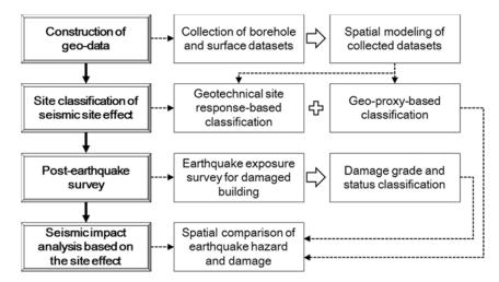
**Figure 2.** Post-earthquake survey framework for rapid earthquake damage estimation correlated with seismic site effects.
