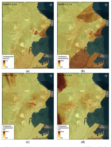
**Figure 5.** Geospatial grid information of representative geo-layers: (a) fill layer; (b) alluvial soil; (c) weathered soil; (d) weathered rock.
