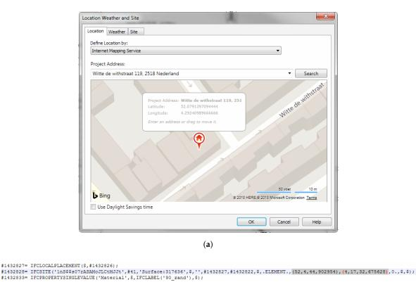
**Figure 16.** Correcting the location of the Witte de Withstraat model. (a) Setting in correct location in the Internet Mapping Service tool; (b) The new coordinates in the IFC file.
