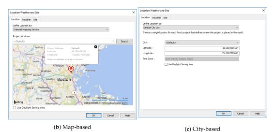
Figure 13. Tools to select a project's location in Revit 2018.
