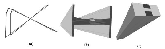
**Figure 6.** Some of the errors present in the test IFC files. **(a)** A prismatic polyhedron with an obvious self-intersection. The self-intersecting top and bottom faces of the polyhedron are not shown. **(b)** A self-intersecting representation of a beam. **(c)** A topological manifold that contains non-obvious geometric intersections. The bottom of the polyhedron, seemingly composed of three rectangular faces, actually has only two rectangular faces that overlap along the middle third.
