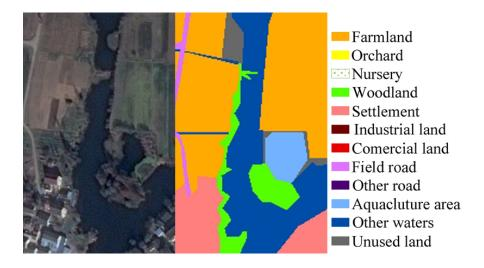
**Figure 2.** An example of a result from the local field surveys. The left picture is a remote sensing image displaying a base map in a field survey. The right picture is a digitalized map showing local land use. The small woodland patches along the river and around settlements could be accurately identified, and areas of aquaculture could be distinguished from other waters through local field surveys.
