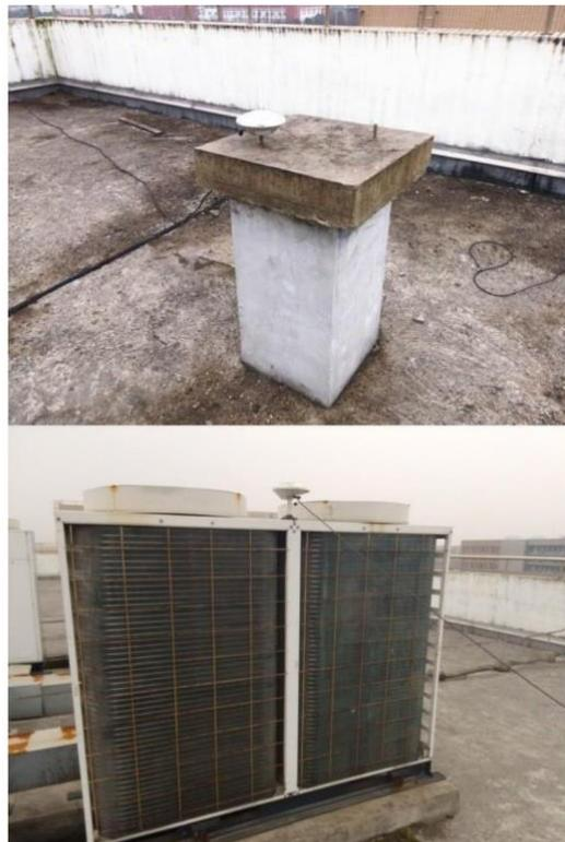
**Figure 1.** Surrounding conditions of the GPS receiving antennas (Photos from Dong et al. [19]). The position of the antenna shown in the upper panel is (31.035631° N, 121.444421° E), and the one in the bottom panel is located at (31.035640° N, 121.444550° E).
