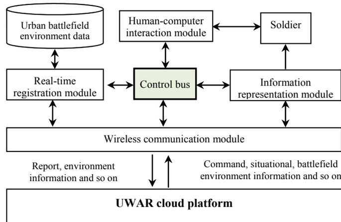
Figure 1. The architecture diagram of Urban Warfare Augmented Reality (UWAR).
