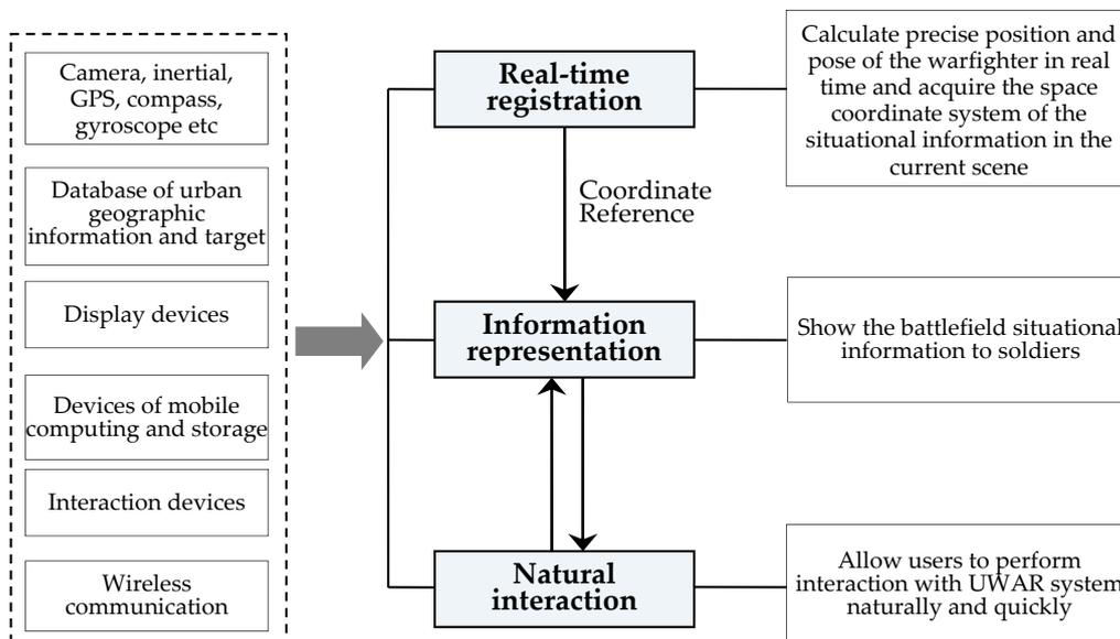
Figure 2. The composition of the three key technologies of UWAR.
