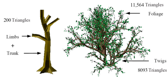
Figure 1. Graphics-based method (200 triangles for the solid part, i.e., trunk and limbs, and 19,657 triangles for the sparse part, i.e., foliage and twigs, by Jakulin [15]).
