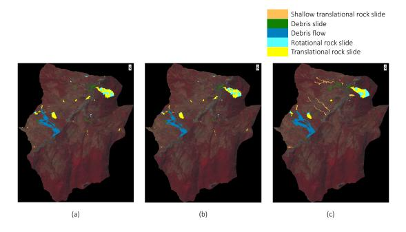
**Figure 6.** Landslide classification (**a**) results from the non-ontological method; (**b**) results from the ontological method; (**c**) ground truth.
