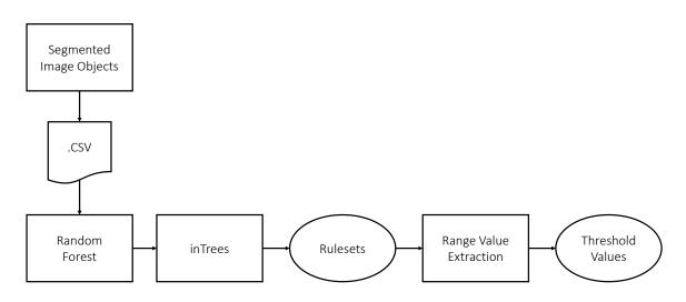
Figure 5. Workflow process for rules threshold extraction.
