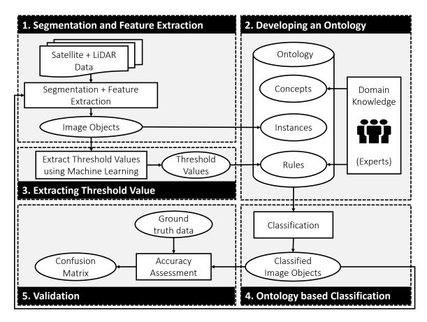
**Figure 2.** Workflow diagram for ontology based image classification with 5 modules; Module (1): Segmentation and Feature Extraction; Module (2): Developing an Ontology; Module (3): Extracting Threshold Value; Module (4): Ontology based Classification; and Module (5): Validation.
