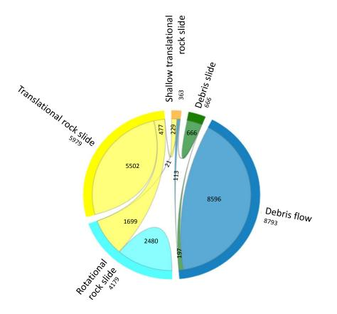
**Figure 8.** Confusion matrix result represented in chord diagram to display the inter-relationships between different landslide classes.
