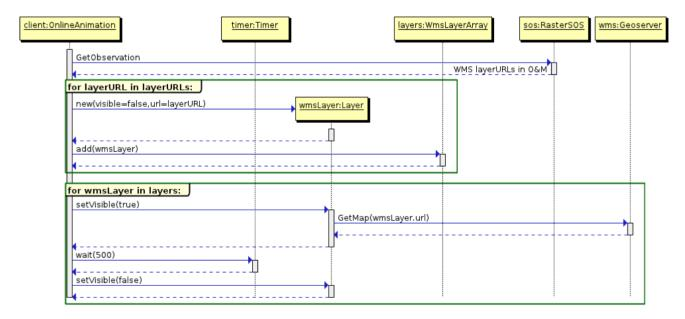
Figure 10. UML diagram of the communication between client, SOS, and WMS.
