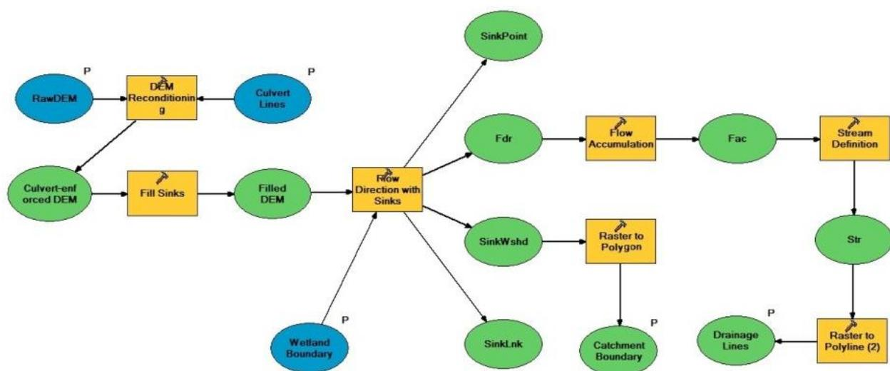
The above processes (Steps 1–7) were automated as a workflow in a ModelBuilder environment within an ArcGIS platform (Figure 2). ModelBuilder streamlined the processes and thus saved the execution time of running each function manually. Finally, the simulated catchment size, drainage channels and depression storage volumes resulting from the LiDAR-derived topography DEM and from the LiDAR-derived hydrologic DEM were compared based on our proposed method.
