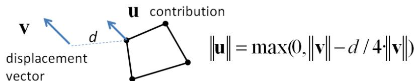
The second constraint is very similar to the first one as the constrained features and vertices are the same. The difference lies in the way the contribution norm is computed (Equation (7)), which absorbs more quickly the displacements. This constraint is preferred to the first one when the positional shift between datasets is large, as it avoids unexpected deformations.
