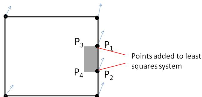
For the additional objects that are not topologically connected to features conflated by least squares (*i.e.*, features inside or near conflated features), a propagation is computed as in Figure 9 on the centroid of the features. Then, the features are simply translated using the centroid propagation, preserving their initial shape.
