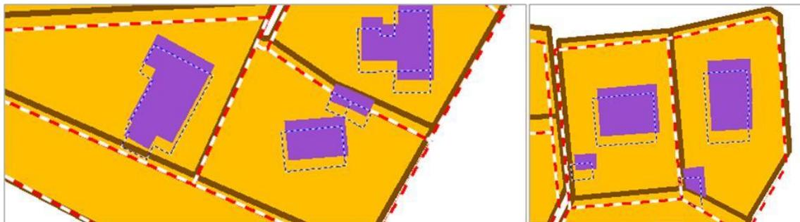
**Figure 21.** (1) Comparison of the least squares based conflation (in plain colors), the rubber sheeting conflation (with dots) and the initial data (with dashes); (2) a broader view of the initial data with deformation vectors.
