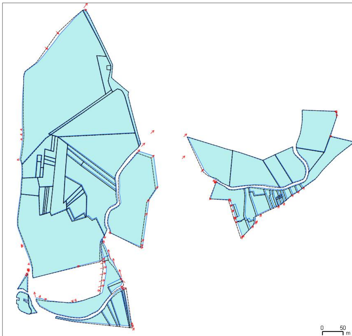
Figure 19. Propagation of the least squares conflation to buildings inside parcels: Initial geometries drawn with dashed lines.
