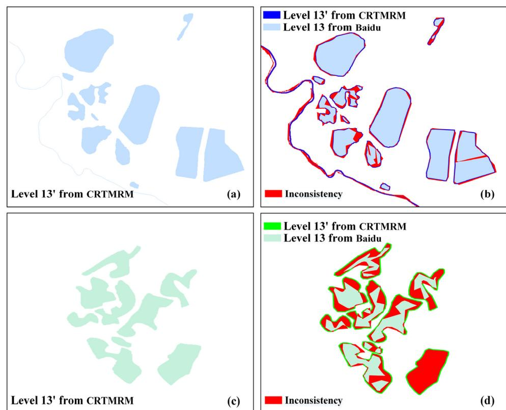
**Figure 13.** Water and vegetation data derivation and inconsistency detection for cross-layer tile maps. (a,c) are water and vegetation at Level 13' from CRTMRM, respectively. (b,d) are the comparison results.
