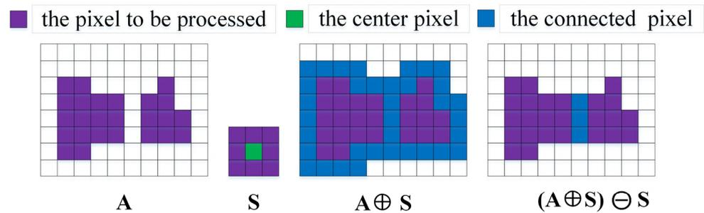
Figure 4. The fracture region connection with the closing operation.
