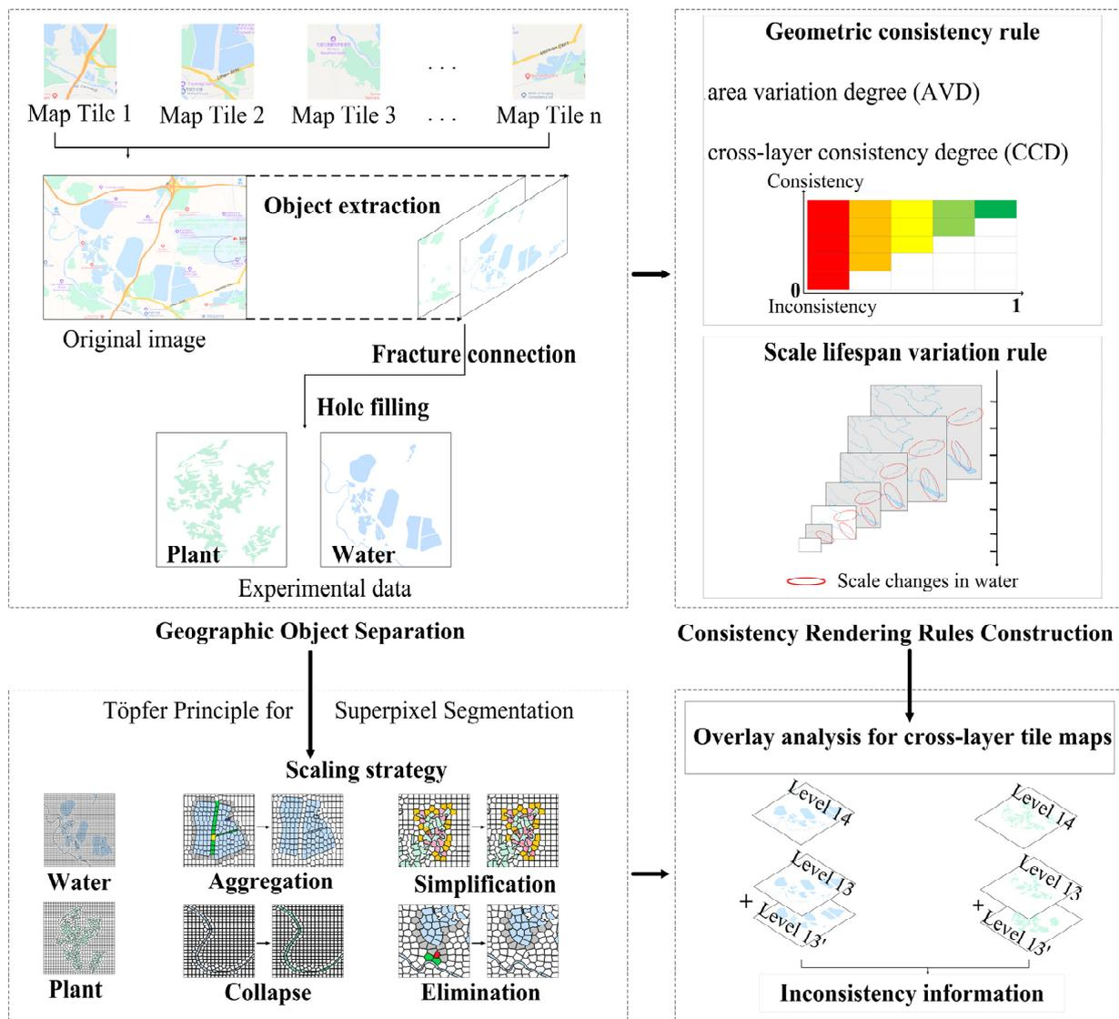
Figure 2. A cross-layer raster tile map rendering method (CRTMRM) for data inconsistency detection.
