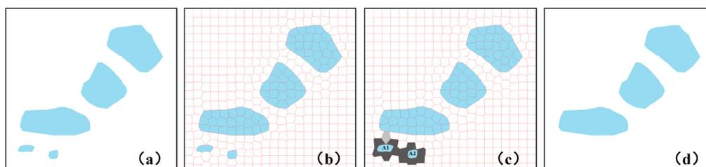
**Figure 10.** The elimination of small areas with the super-pixel: (a) original data; (b) super-pixel segmentation by SLIC; (c) the classification and selection of small areas; (d) the result of elimination.
