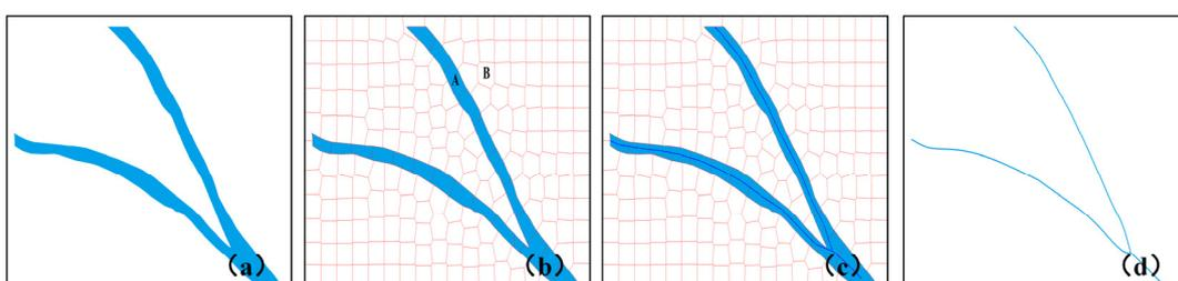
**Figure 8.** The collapse of bilinear river with the super-pixel: (a) original data; (b) super-pixel segmentation by SLIC; (c) the centerline extraction from the super-pixels; (d) the result of collapse.
