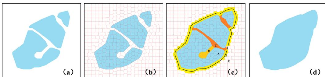
**Figure 7.** The lake aggregation with the super-pixel: (a) original data; (b) super-pixel segmentation by SLIC; (c) the classification and selection of different super-pixels; (d) the result of aggregation.
