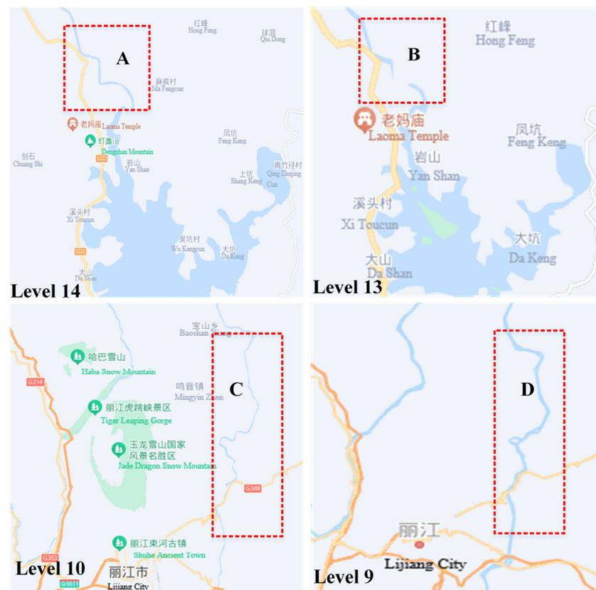
**Figure 1.** Inconsistencies during the tile map rendering at different levels. (A,B): river breakage in low-level representation; (C,D): overlapping rivers.
