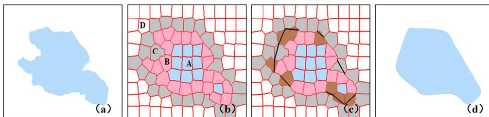
**Figure 9.** The simplification with the super-pixel: (a) original data; (b) super-pixel segmentation and the classification by SLIC; (c) the selection and the bend smooth from different super-pixels; (d) the result of simplification.
