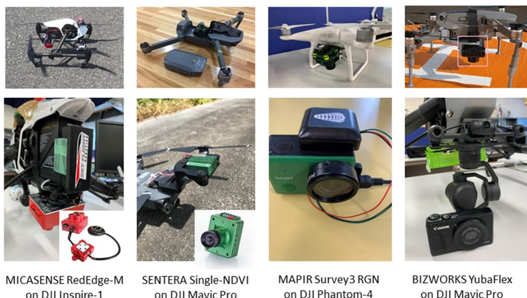
**Figure 3.** Multispectral cameras used for this analysis.
