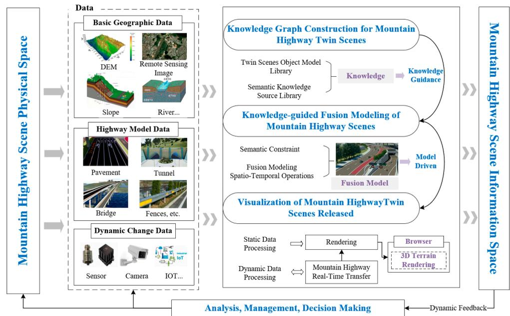
**Figure 1.** A general framework of the knowledge-guided digital twin scene fusion representation method for mountain highways.
