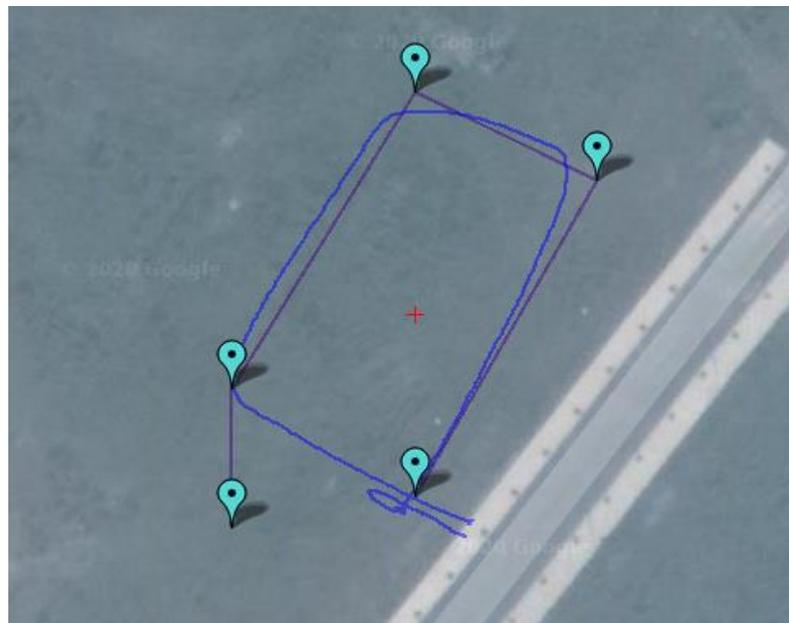
**Figure 20.** The difference between desired and real trajectories (pink line—desired trajectory, blue line—real trajectory).
