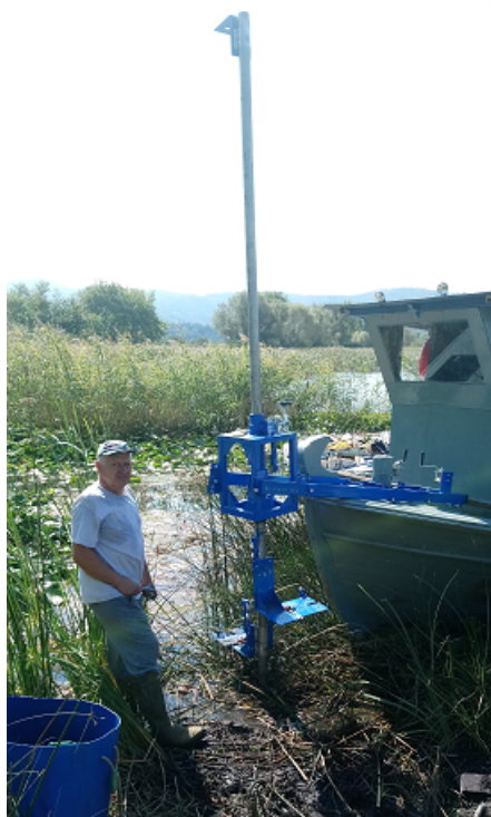
Figure 6. Supporting infrastructure for the acquisition of GPS and hydroacoustic measurements.
