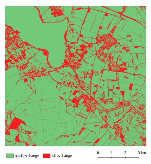
**Figure 7.** Monitoring class mismatch between the original cadaster data and the LightGBM prediction to visually assess the results of the classification. Sources: Sentinel-2 imagery from 30.3 to 16.10.2019 [80], Czech cadastral map [85].
