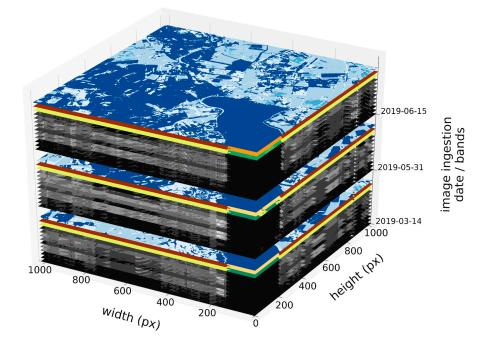
**Figure 3.** Merged features (three sample multi-image features on the top of bands) stacked in time as the result of the MergeFeatureTask. By this time, they are already filtered by thresholding respective SCL masks (see Section 3.2.7).
