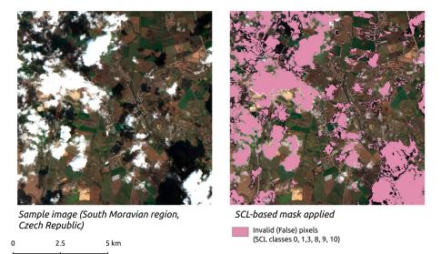
**Figure 2.** Sample scene classification layer (SCL)-based mask applied on a Sentinel-2 image. Data source: Sentinel-2 image from 14.3.2019.
