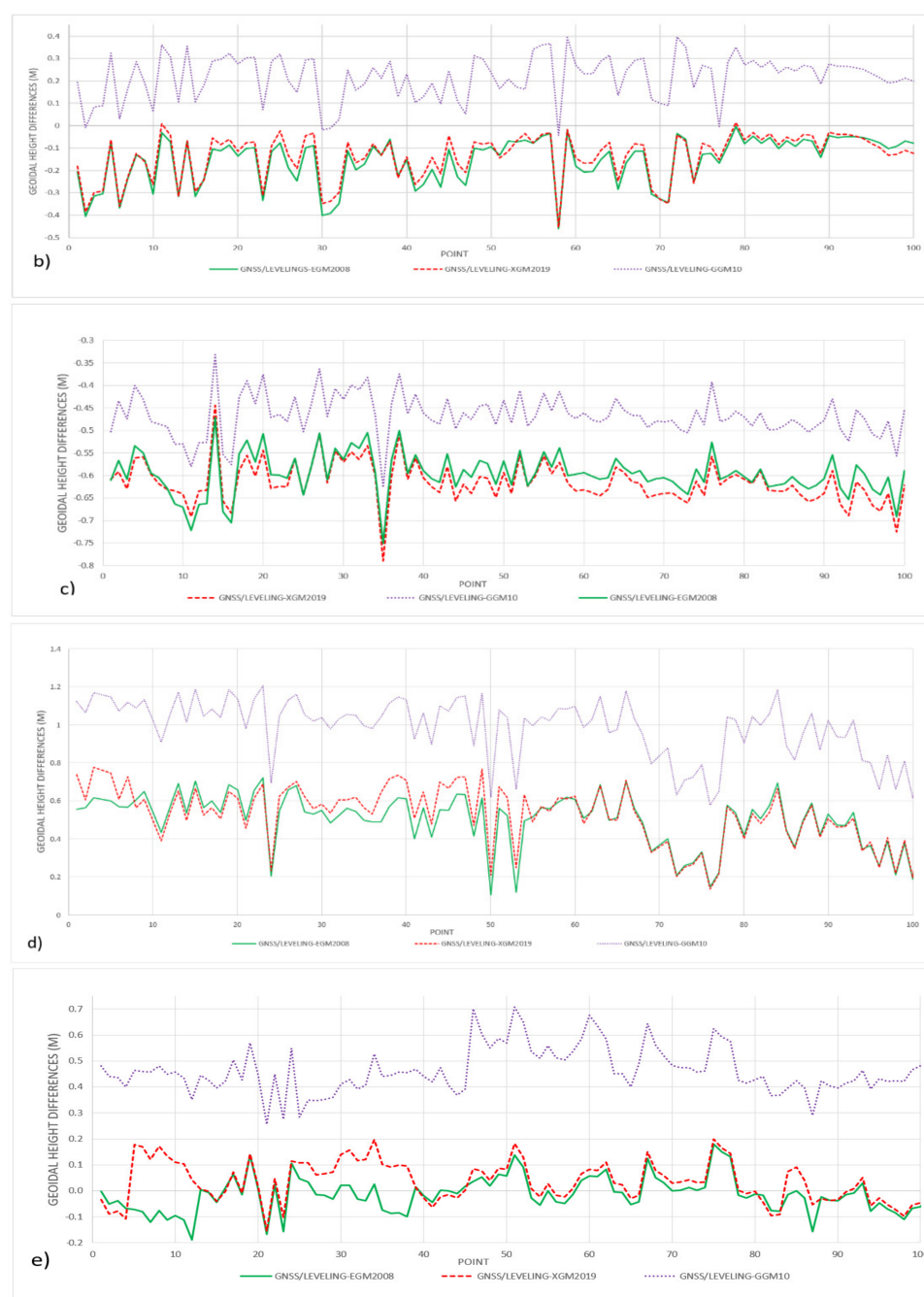
Figure 2. Geoid undulation differences between the geoid models: EGM2008, XGM2019e_2159, and GGM10, and GNSS/leveling stations for five Mexican urban areas: (a) Durango, (b) Hermosillo, (c) Merida, (d) Mexico City, (e) Monterrey. Units: Meters.
