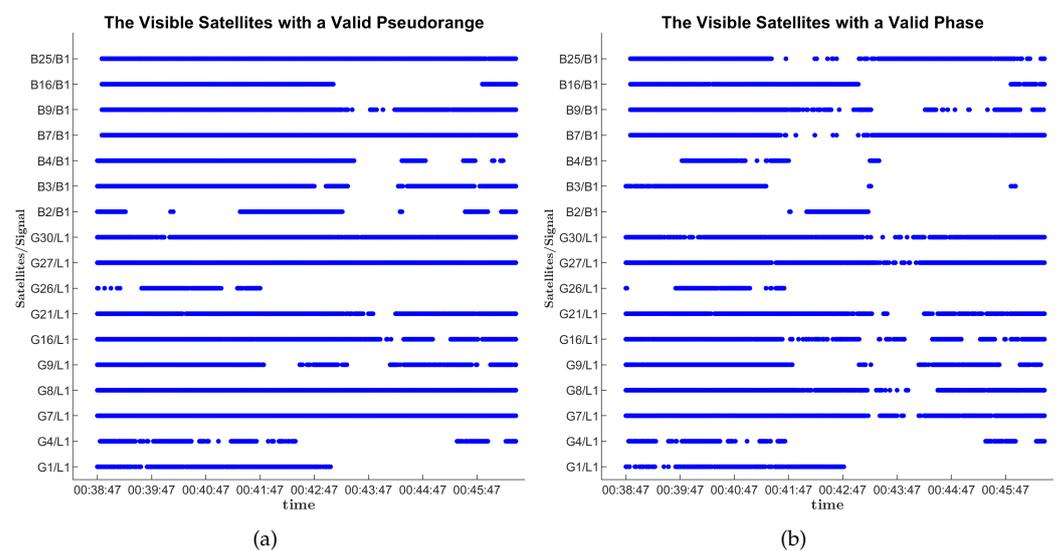
**Figure 10.** The visible satellites with a valid pseudo-range and the visible satellites with a valid carrier phase. (a) The visible satellites with a valid pseudo-range. (b) The visible satellites with a valid carrier phase.
