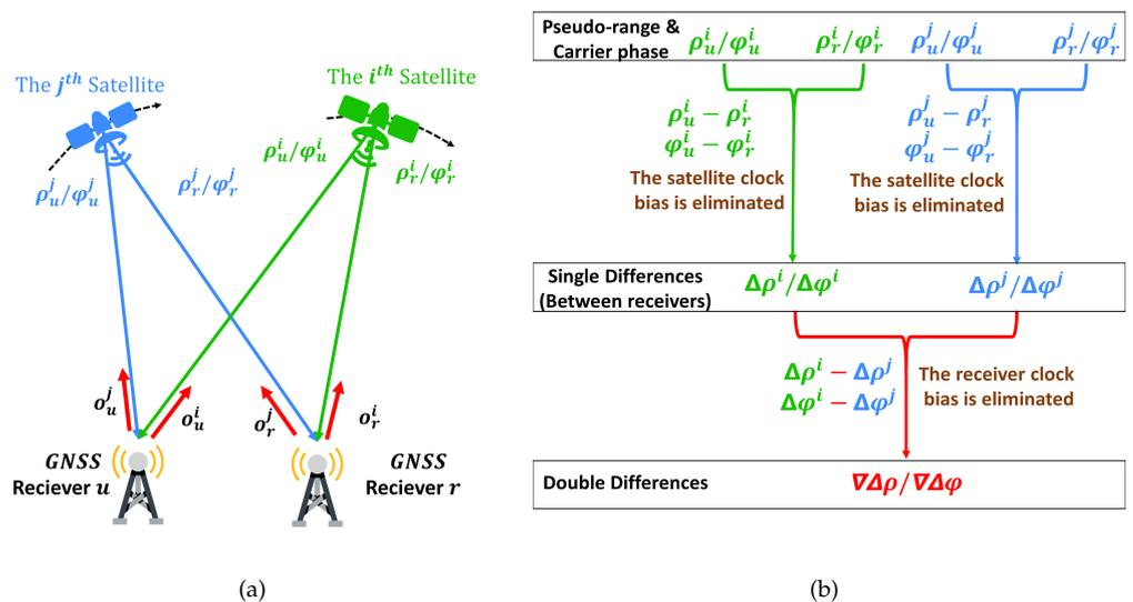
Figure 2. SD measurements and DD measurements. (a) Two receivers track the signals of two satellites. (b) Steps to calculate SD measurements and DD measurements.
