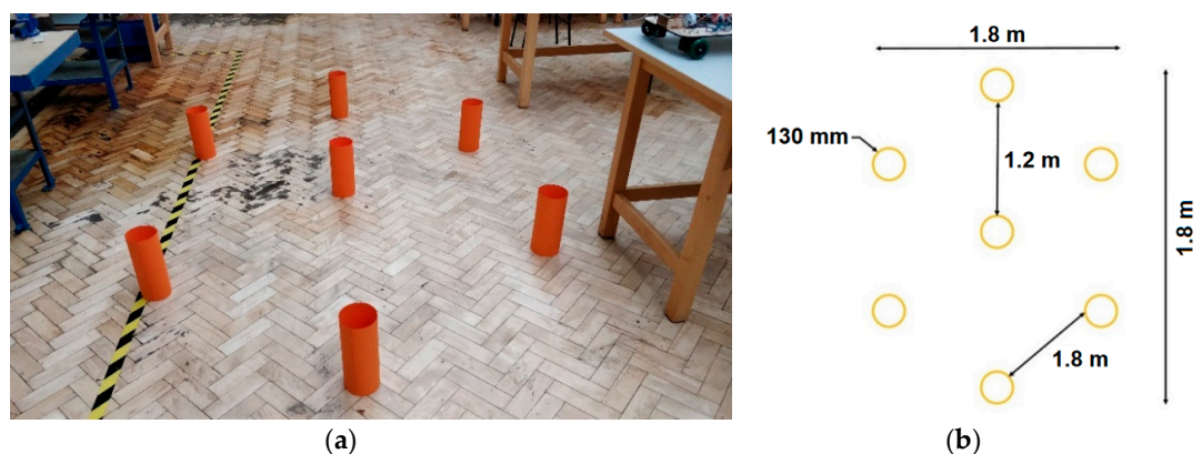
Figure 5. (a) The lab obstacle course, and (b) corresponding dimensions for this course.
