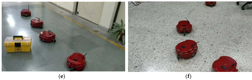
Figure 8. Chaining behaviour of robot. (a) Starting position of the robots; (b) The initial motion of the robots; (c) The robots intelligently avoiding an obstacle; (d) The robots staying together and avoiding a dynamic obstacle placed in the way; (e) Robots after successfully avoiding the obstacle; (f) Robots reached the goal.
